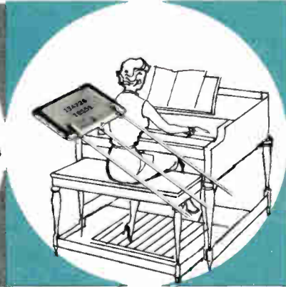
ELECTRONIC ORGAN — PEC filter reduces sharp transient of keying to give natural touch response.
