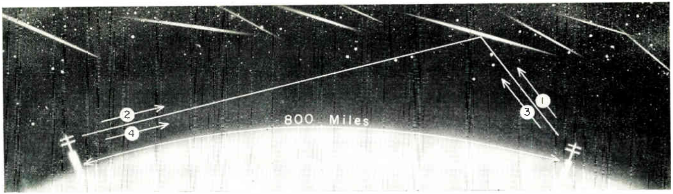
Fig. 24: Meteor-Burst operational sequence: (1) constant VHF beam from receiving station, (2) notice from receiving station to start message transmission, (3) message transmittal, (4) message-termination signal from receiving station.
