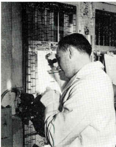
Fig. 3: Processed microfilm is closely inspected for scratches as it leaves the drying cabinet in the Recordak laboratories.
