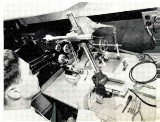
Fig. 6: Jeweler's lathe and microscope are used to grind pivots for gimbals mounting
