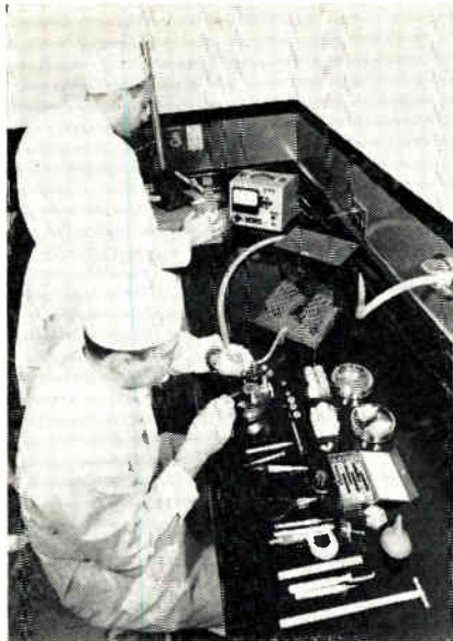
Fig. 1 left: Technician in foreground is making a "float" assembly while the other one inspects a completed assembly. Gyro is "floated" in a viscous fluid to absorb friction and shock.
