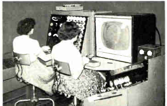
Sylvania tubes undergo arc tests in TV receiver circuits as part of its extensive Dynamic Testing Program.
