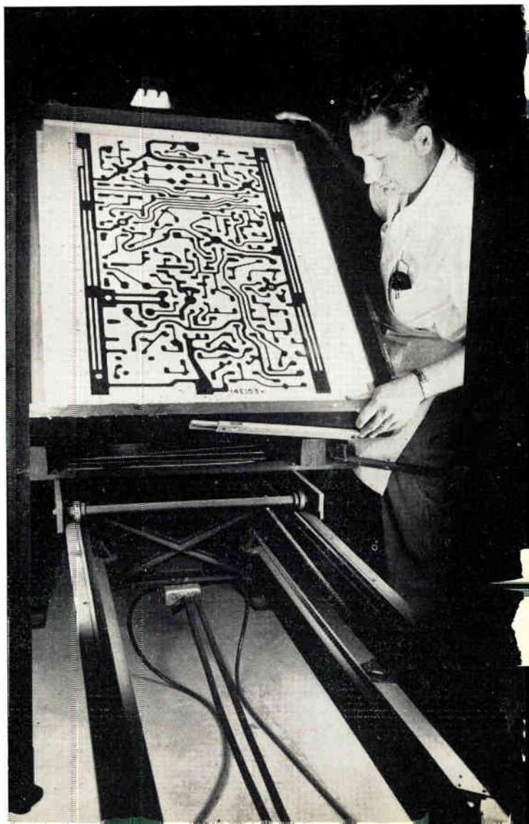
Fig. 2: First step is photographing a large drawing of the ckt.
