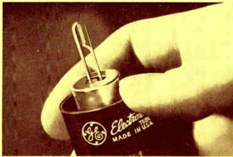
ABOVE: a special tungsten post shields G-E tube filaments from electrostatic pull of high anode voltages. BELOW: checking 1B3-GT and 1X2-A/B rectifier types during G-E flyback life test that further safeguards tube performance.
