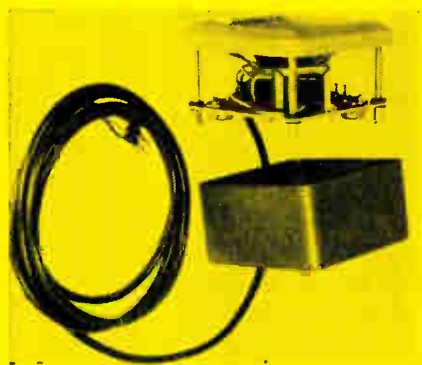
Transistorized speaker unit boosts mobile radio output to overcome vehicle noise
