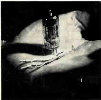
Fig. 1: Tube, transistor, and cryotron—two twisted wires form new computer element
