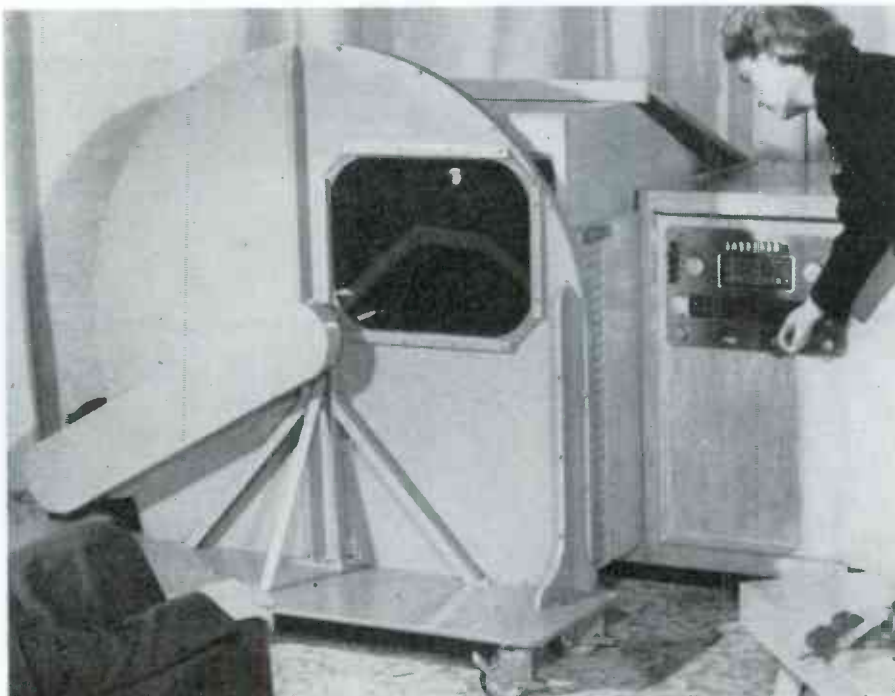
Fig. 3: DuMont's showing of a "converter" for CBS color designed for receiver with a 19 in. tube, while a stunt, must have impressed observers with unwieldy impracticality of such a mechanical disc. The converter is about 5 ft. high and weighs about 700 lbs.
