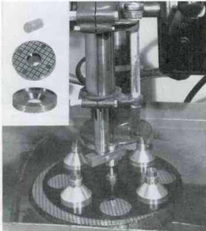
(Left) Recently developed inkwell apparatus permits easier inspection of individual quartz crystals as they are ground. Inset shows an unassembled view of the lapping apparatus
