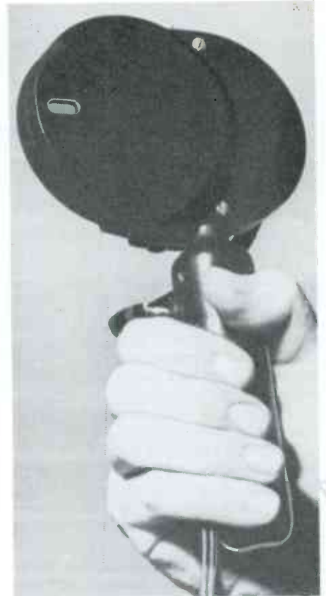
Fig. 4: CBS hand-held color converter. Unit contains a small three color disc driven by a synchronous motor and makes it possible to receive color pictures on a monochrome receiver modified to receive the new scanning frequencies. A simple change in the receiver scanning circuits, controlled by a two-position switch, adjusts operation to either color or monochrome standards
