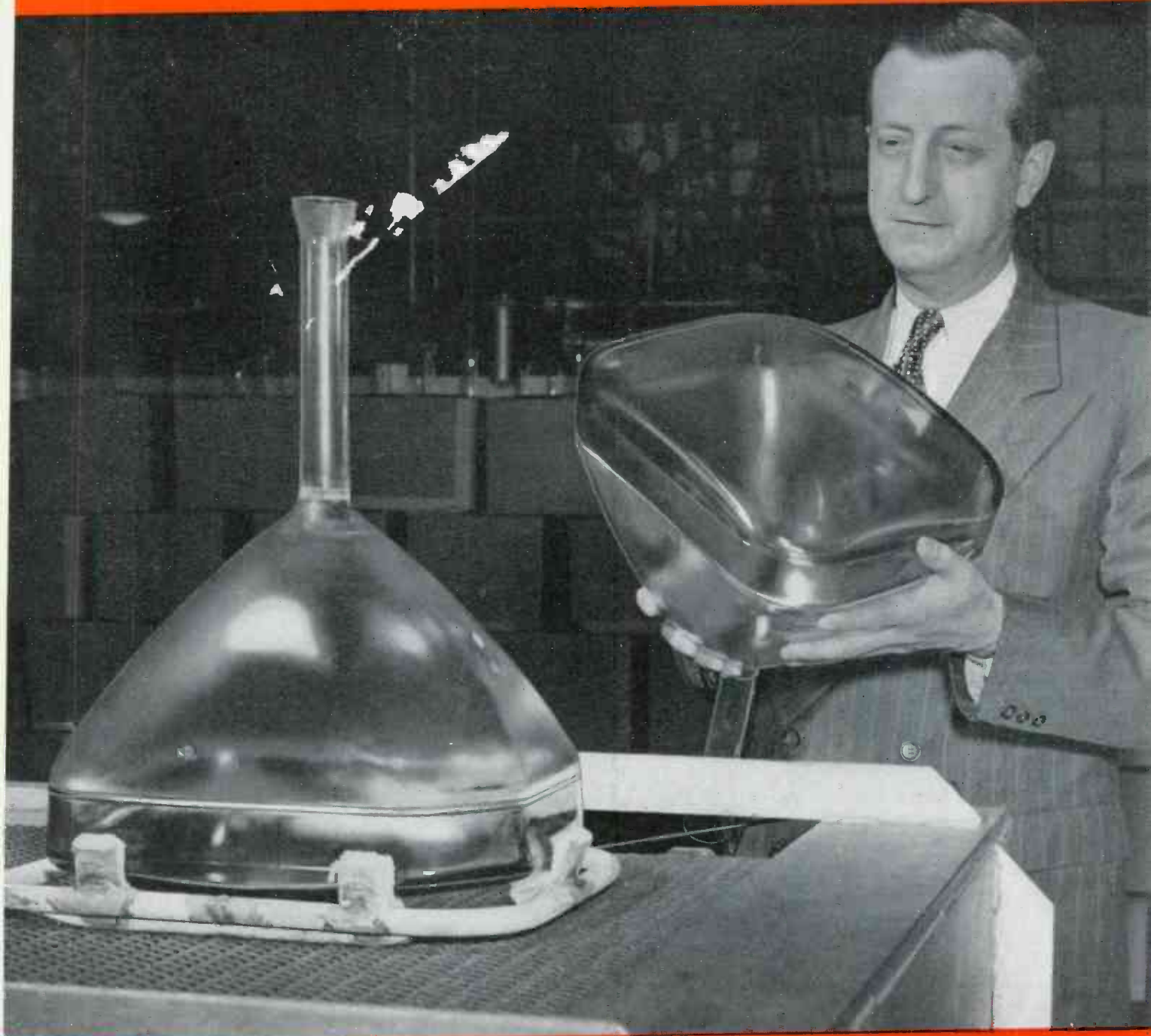
Photo: Dr. Harvard B. Vincent, Director of Product Development, American Structural Products Co., Toledo, Ohio, inspects face plate of a new 16-in. oil-glass rectangular television bulb. The bulb at left is emerging from an annealing lehr on a special asbestos carrier.
