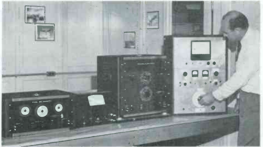
Fig. 10: Four phase measuring units developed for use at Consolidated Vultee Aircraft Corp.
