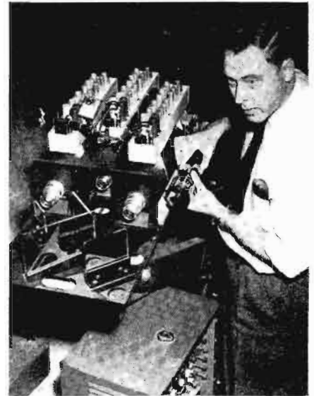
Fig. 1. Three tube RCA color camera demonstrated by Richard Webb, RCA engineer
