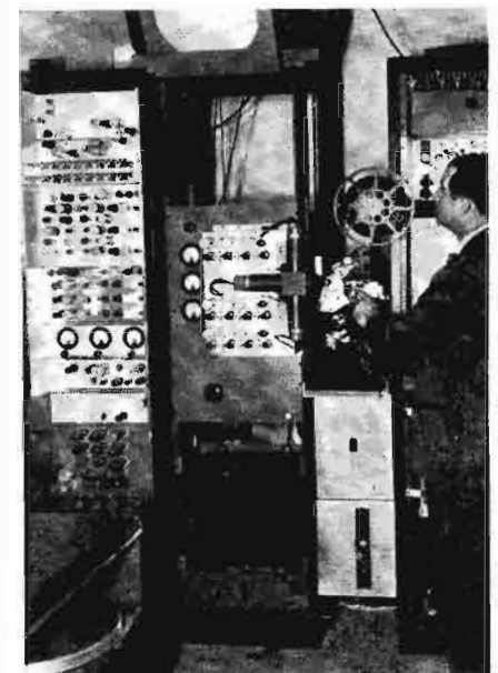
(Left) RCA projection set uses three kinescopes, reflective optics, and a pair of dichroic mirrors to produce color pictures (Below) Three tubes are required for full color pick-up from the 16 mm projector. The electronic sampler unit is shown at left
