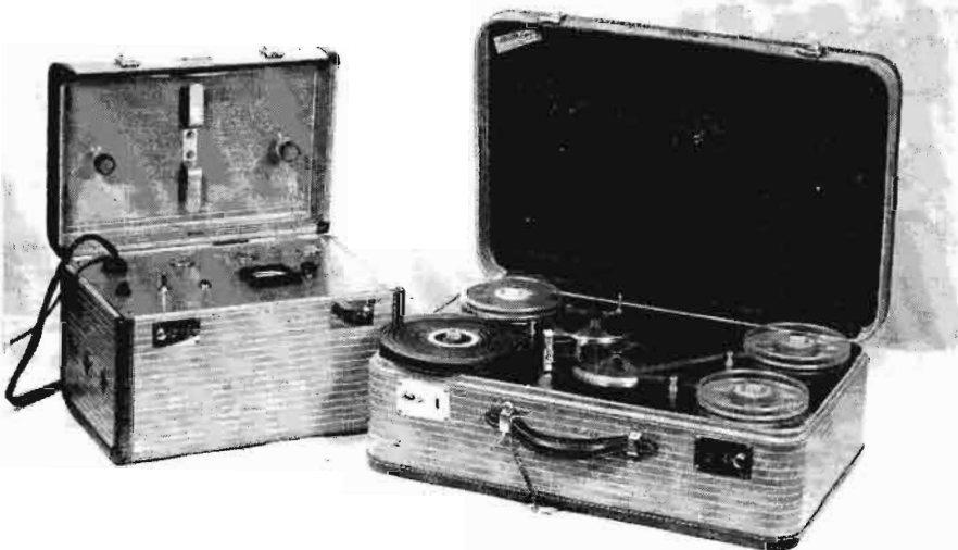
Fig. 4: Portable demonstration duplicator. Tape speed is about 20 in./sec. with a 2 KC idealizing frequency. Field is directed transversely with respect to tapes
