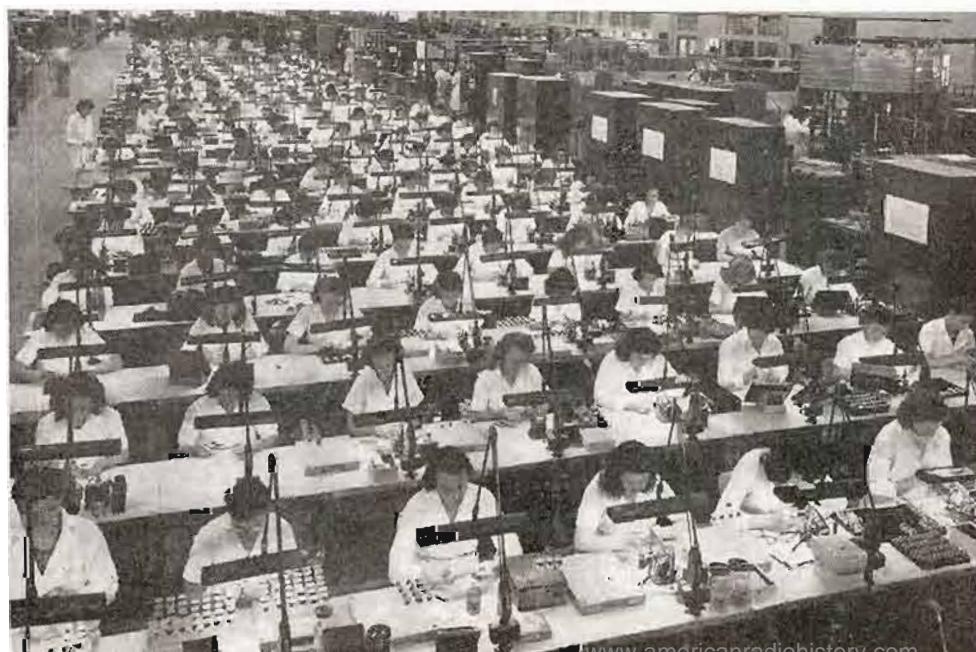
In the miniature tube assembly section, each row operates as a team. So sensitive are these electronic tubes to dust and lint that employees wear special lint-free smocks
