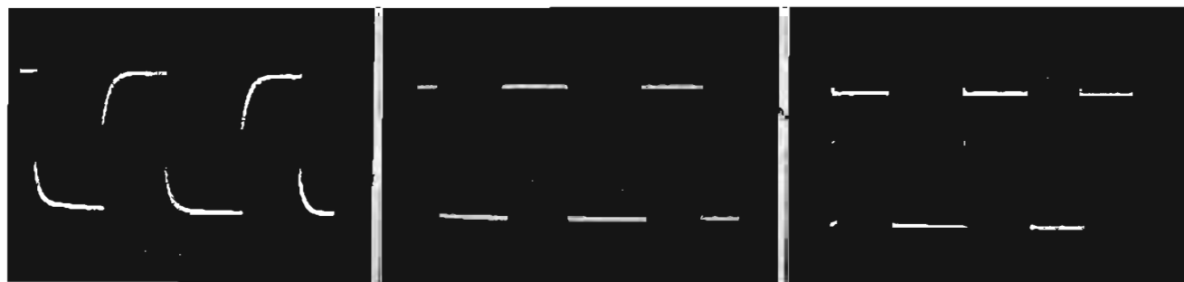
Fig. 2: Oscillograms showing response of three amplifiers represented by A, B, and C respectively (Fig. 1) to a square wave signal
