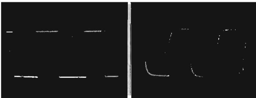
Fig. 3: Maximum (left) and reduced (right) gain control effects upon amplifier bandwidth
