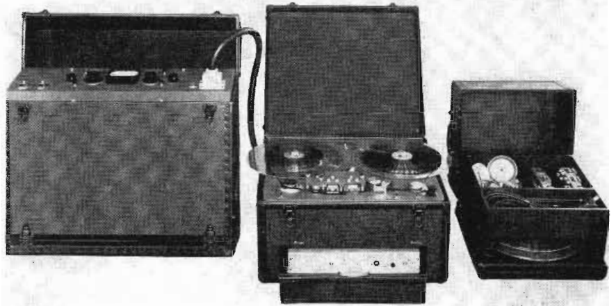
Fig. 2: Portable unit showing amplifier on left, tape unit in center and spares on right
