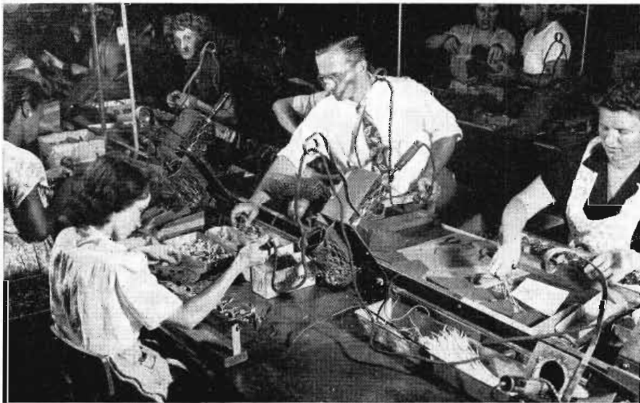
ABOVE: Operations at Emerson begin with component parts assembly. Condenser and resistor leads being cut to size at 900-per-hour rate
