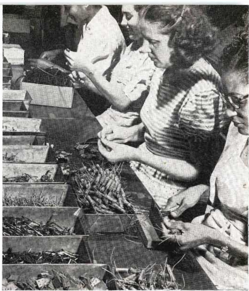
ABOVE: Operations at Emerson begin with component parts assembly. Condenser and resistor leads being cut to size at 900-per-hour rate
