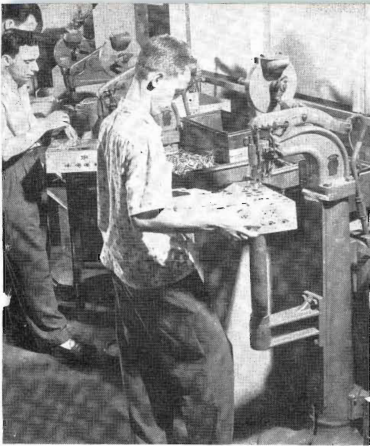
ABOVE: After assembly of component parts, they are riveted to the chassis. Operation includes 23 tube sockets, 8 electrolytic condenser plates, 5 insulators for control units, 2 output transformers
