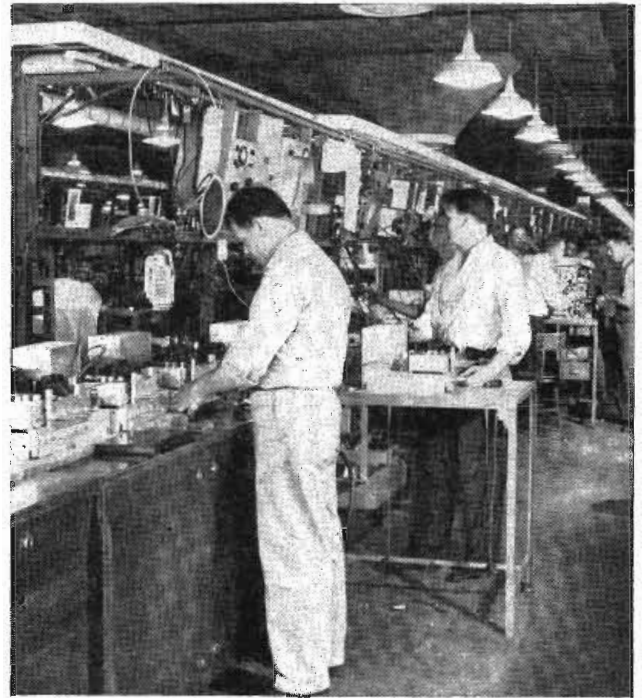
ABOVE—At end of test section where chassis are checked for continuity after wiring, they are aligned and performance tested. Note use of incandescent lights; fluorescents cause interference.
