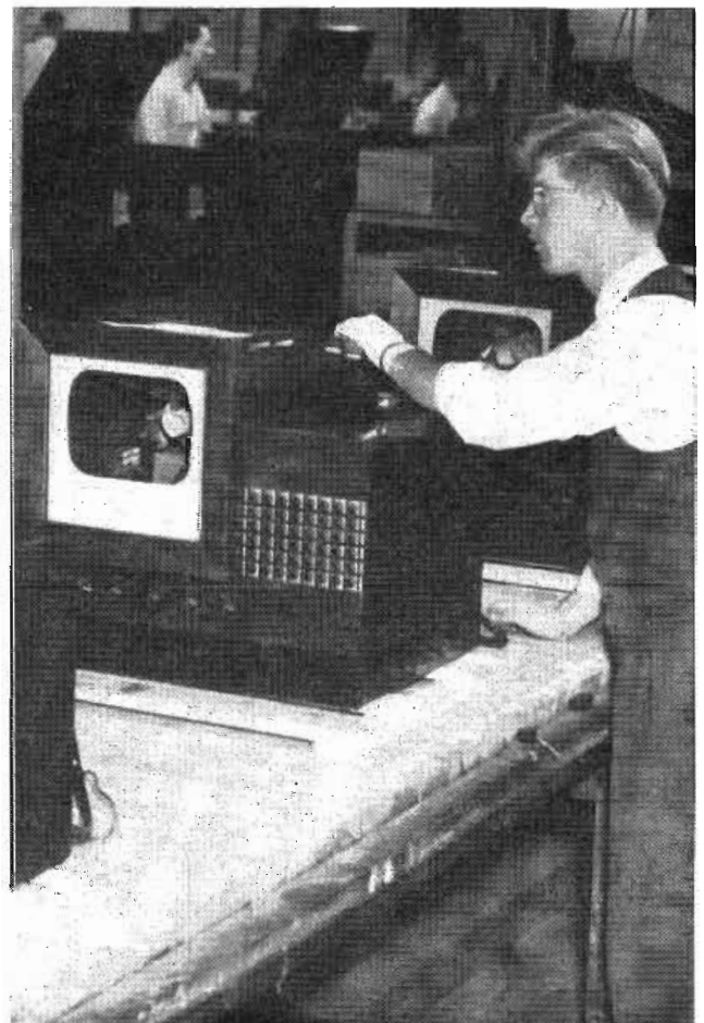
BELOW—First step in the insertion of chassis into receiver cabinet. Finished job is packed as shown in large photo on page 36.
