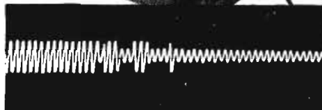
Plot made on Type 314 of starting current of small synchronous motor. (Note variation in current as the rotor "hunts" for its synchronous speed).
