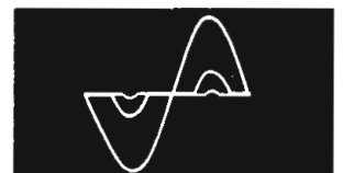
Triple exposure made with Type 271-A while varying constants of peak-clipping circuit.
