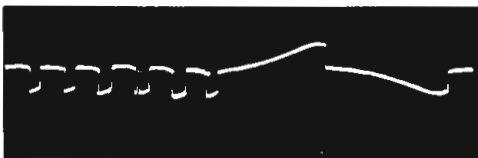
Output voltage of Type OB2 Voltage-Regulator Tube, with sudden applications of resistive load, using Type 314 Continuous-Motion/Single-Frame Camera.
