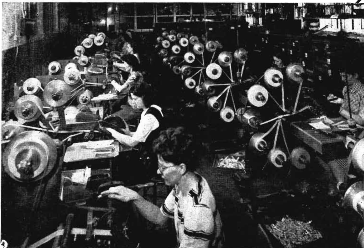
Skilled operators rolling fabricated plate electrolytic capacitors.
