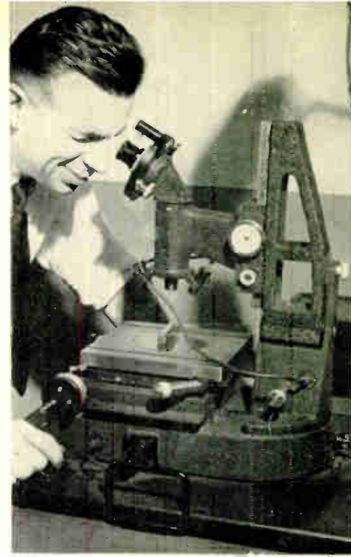
To maintain accuracy with this toolmaker's microscope, the temperature in this room is controlled within extremely close limits
