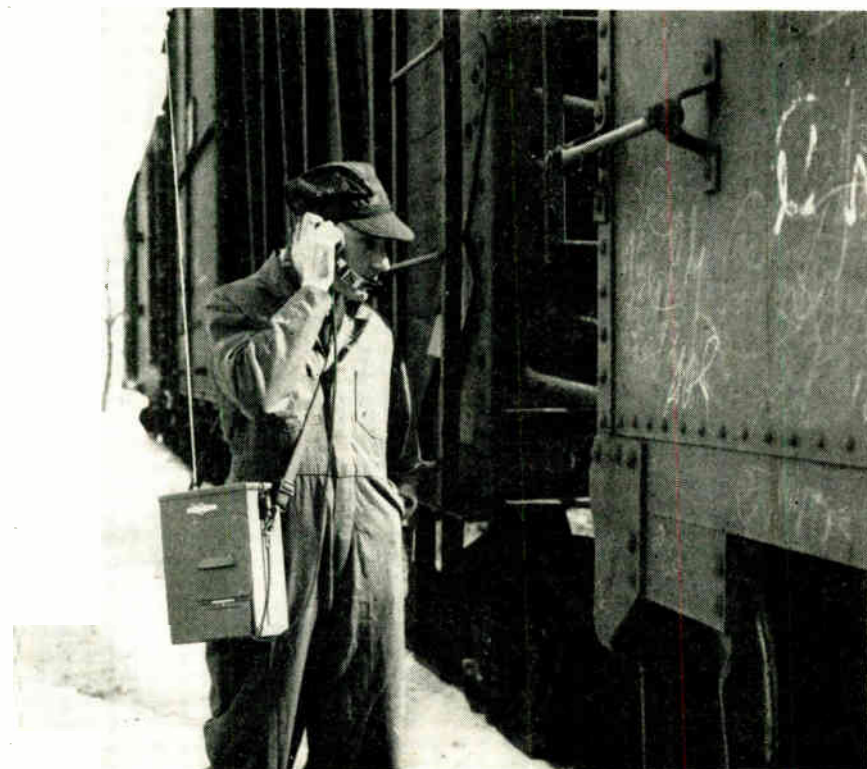
Bendix MRT-2B VHF FM railroad radio pack set provides trackside extension of standard VHF communications for railroad use
