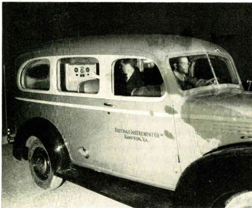
Master station installed in carryall for field operations
