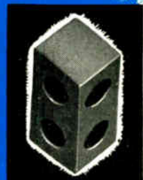
LONG-LIFE combination fuse-holders and pullers of "Buna-S" synthetic rubber. One end, which is stored red, faces panel when both "working" and "spare" fuses are good, is exposed when holder is turned to insert spare. Available for 3AG, 4AG and 5AG size fuses.
