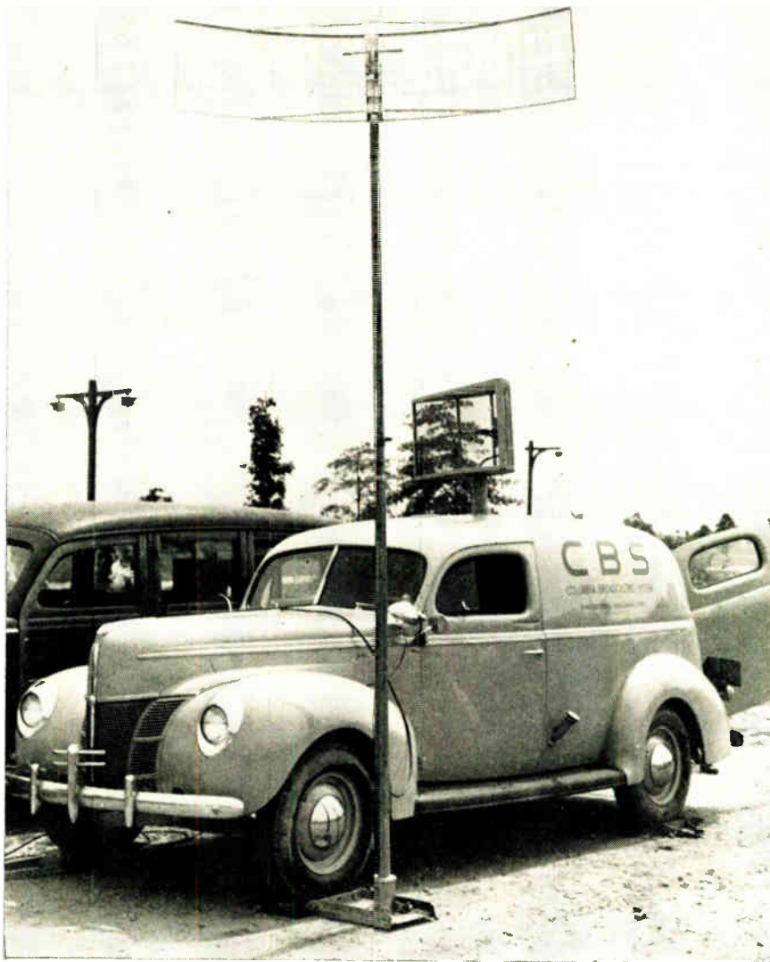
Field equipment ready for UHF television tests showing parabolic receiving antenna on field car and on twelve foot pole
