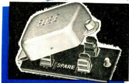
STEEL COVERED 3AG size fuse mountings available in single and double pole types, and in single pole and spare fuse holder combinations, with hinged cover; also in double pole types with removable non-hinged cover.
