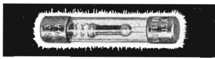
SLO-SLO 3AG Littelfuses have high time-lag to withstand heavy surges—quick on shorts. Anti-fatigue construction. In 1/100 to 20 amp. ratings.
