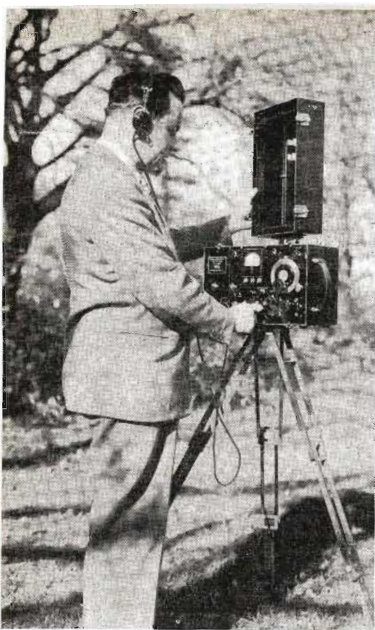
Field intensity meter in use, with operator adjusting loop for maximum rating
