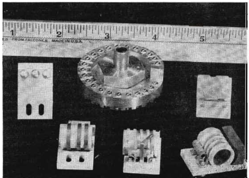
Fig. 3—The tank circuit in detail, showing various parts described in the text. Tuning slugs for coils are advanced by positioning of axial cam at center.
