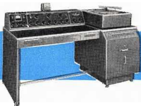
1939. This custom-built audio console for WOR was the first commercial type meeting all requirements for FM use. It provided circuits and equipment to meet specific operating conditions. The tailored metal desks mounted amplifiers, control and switching equipment and turntable units—all within easy reach of the operator.
