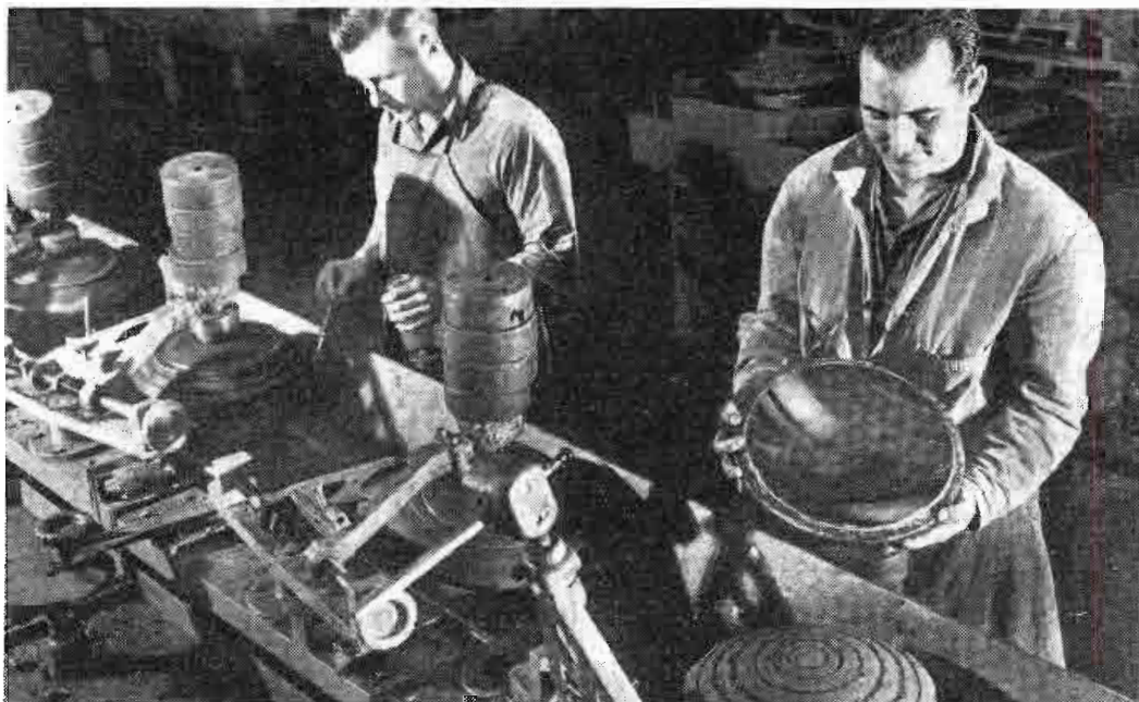
One of the complex processes by which American Optical Co. produces spherical mirrors and correcting lenses which are the basis of many projection systems
