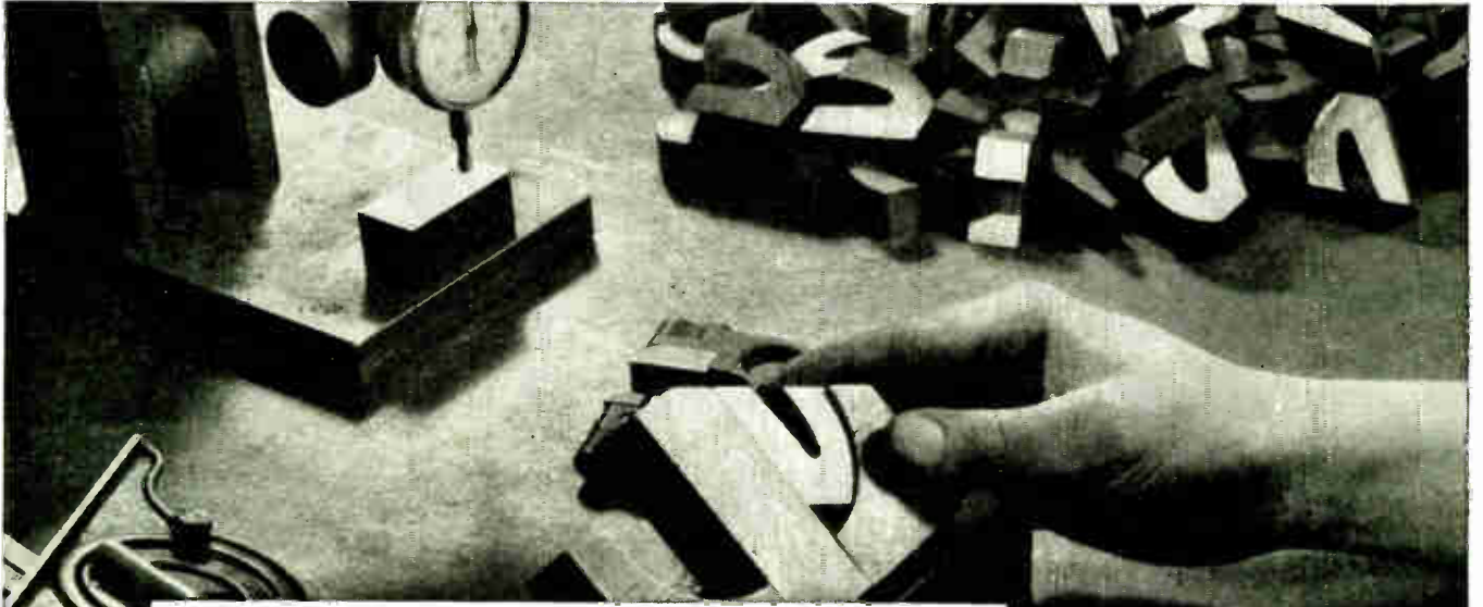
FLUXMETER CLOSED CIRCUIT TEST
