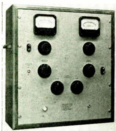
Fig. 1—Panel arrangement of the Model 502 Intermodulation Distortion meter
