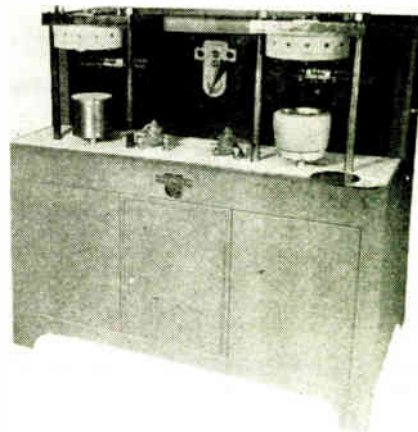
Induction heater for brazing bottom on cooking utensils. 2 place jig provides steady work flow
