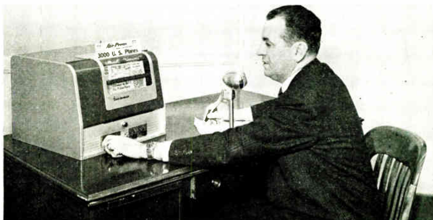
Above, transmitting scanner designed by Finch Telecommunications, Inc. Below, home receiving unit
