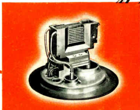
Unusual construction is indicated by this view of the header with filament, grid #1 and grid #2 in position. Precision cast and machined electrodes are connected to water ducts for internal cooling.
