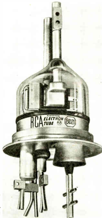
Two views of RCA's new internally water-cooled twin tetrode, complete above, and below, showing header with filament and No. 1 and No. 2 grids in position
