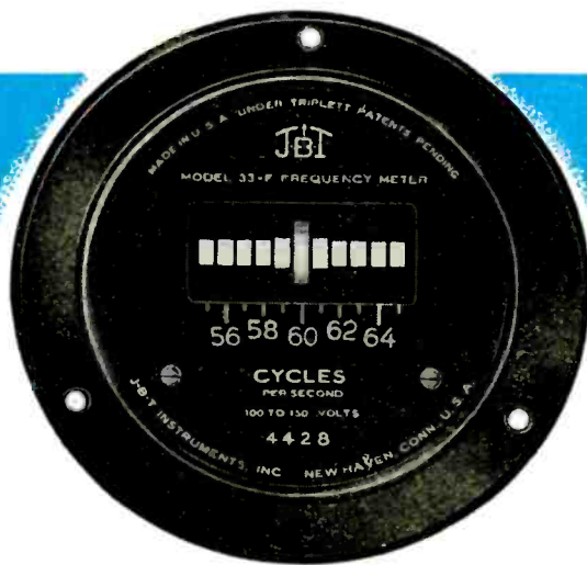
Model 33-F, Full-cycle increment, shown indicating frequency of 60 cycles. Black dial for special application.
