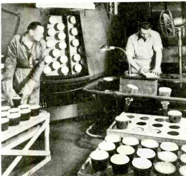
Fig. 15—The bulb is outgassed by heating in an oven at 400 deg. C. Fig. 16—A short aging process stabilizes the finished product.
