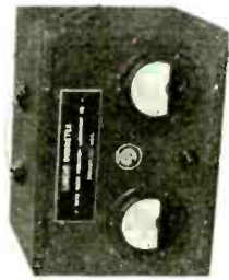
FOR ADDITIONAL OSCILLOGRAPH GAIN PA114 PRE-AMPLIFIER & 150-VOLT POWER SUPPLY.
