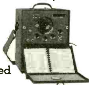
Heterodyne Frequency Meter covering a range of 85 Mc. - 1000 Mc.
