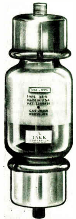
Figs. 4 & 5—Newly developed H V rectifiers; fuse type anode and cathode terminals permit reversing output polarity when required
