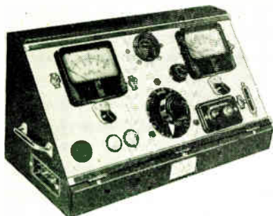
Fig. 10—Control console for Model 48 allowing complete remote control of high voltage output
