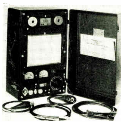
Fig. 1—Self contained, portable model with a dc output up to 15,000 v; insulation readings can be made direct from one dial and chart
