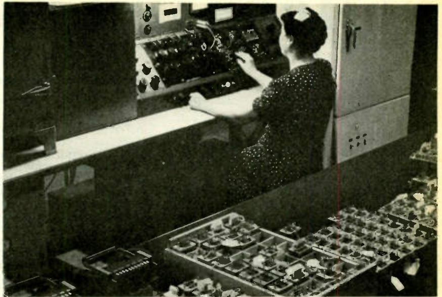
A view of a typical test position where thermistors are individually checked as to a complete series of operating characteristics. These tests are made on complete units consisting of the thermistor, the heater, and compensating networks
