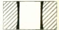
Black area illustrates controlled variation in depth of hardening from .030" to .125", 40-45 Rockwell-C.
