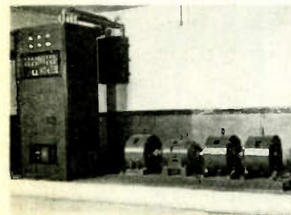
Fig. 2. Motor generator set showing three single phase generators and driving motor
