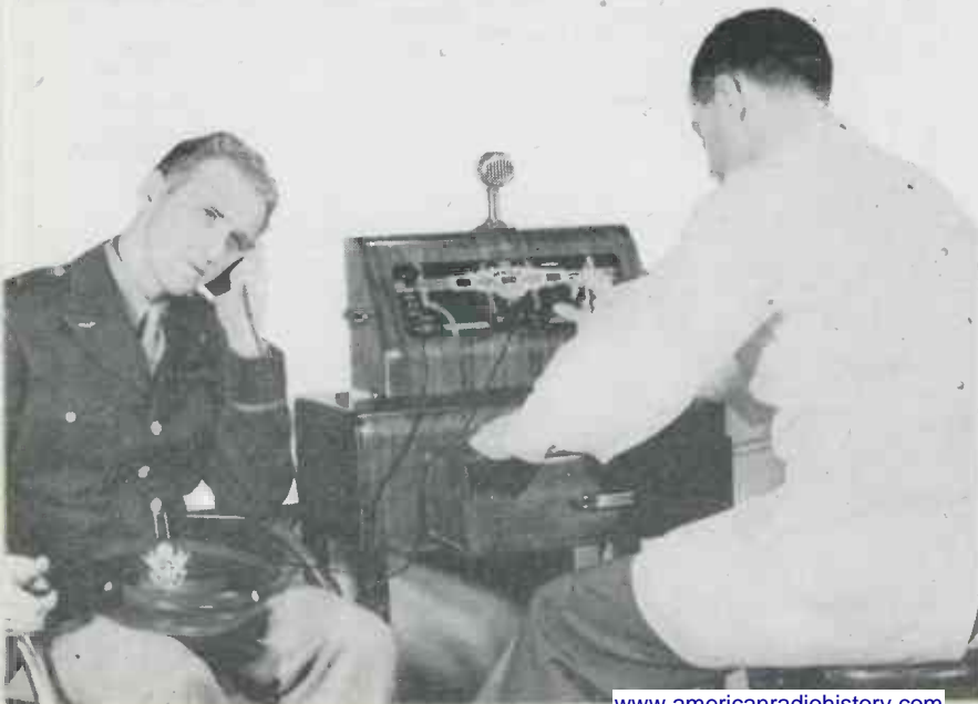
Fig. 4—Practical application of the audiometer which consists of a high stability audio oscillator, a precision wide range attenuator, a low distortion amplifier and a high quality, calibrated headphone transducer.
