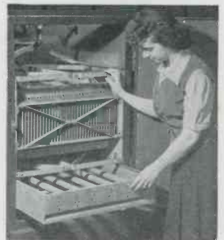
Experimental model of postwar Westinghouse Precipitron for the home eliminates dust rag
