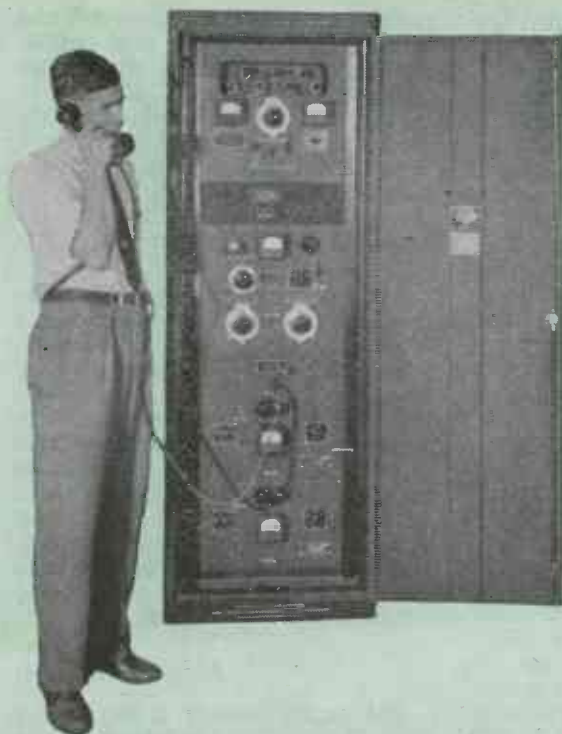
Above—A more compact panel mounted assembly that handles all of usual carrier functions. A typical power line carrier assembly housed in a steel cabinet, containing from top down, a power distributing unit, with the telephone line test jacks, receiver, telephone unit, electronic transfer control chassis, transmitter chassis and, at the bottom behind the screen, the power amplifier chassis
