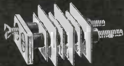
High voltage spring pile-up insulators of special heat- treated Bakelite. Has mini- mum cold flow properties, low moisture absorption content and permits punching without cracks or checks.
