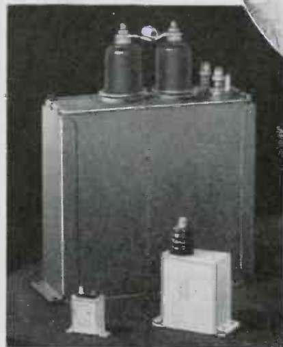
G-E capacitors designed for h-f oscillator circuits. Large unit: high-frequency, parallel-plate capacitor for the resonant circuit. The others: an oil-paper, high-frequency blocking capacitor, and (smallest) a Pyranol by-pass capacitor.
