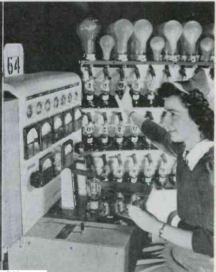
3 —"Trolley Car Test Set" at Westinghouse Lamp Division, Bloomfield, N. J., so named because of the obviously reminiscent control handle, which advances tube to be tested to point where contact is made. Preheating and storage rack at girl's right
