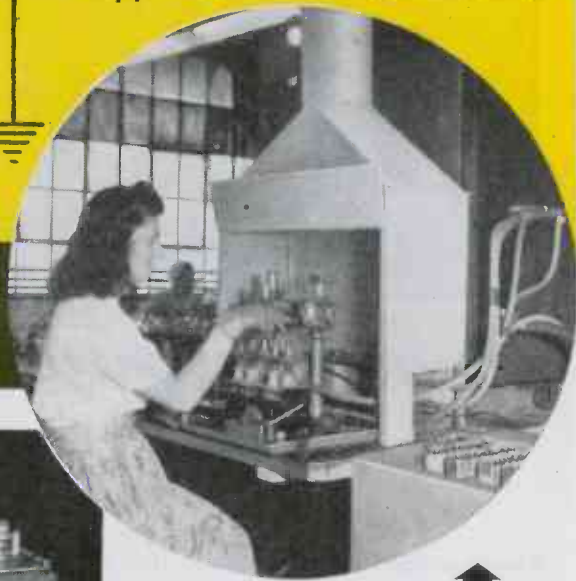
Electronic heater being used to solder on the covers of G-E capacitors. Four units are soldered simultaneously.
