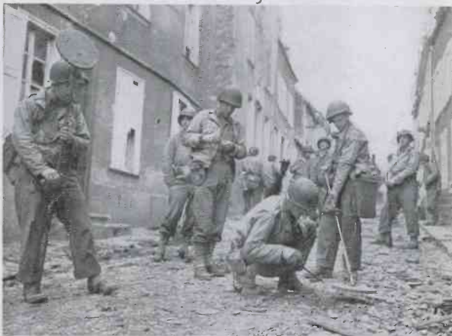
Top—Signal Corps photo showing SCR 625-F mine detector in use under battle conditions as engineers check the ruins of St. Lo for buried explosives. Center—Exploded view of the equipment showing its various components. Bottom—Photographed in North Africa, these three types of German Tellur mines are charged with 11 pounds of explosives
