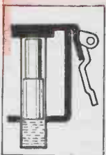
Plunger after overload with armature attracted to pole piece, opening contacts.
