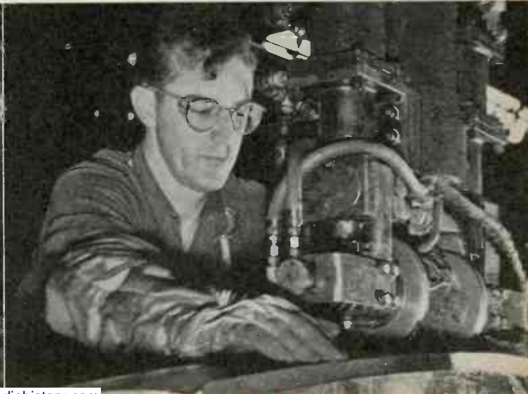
TWO WELDS are made simultaneously in this operation on one of the halves of a tear-drop shape dropable fuel tank
