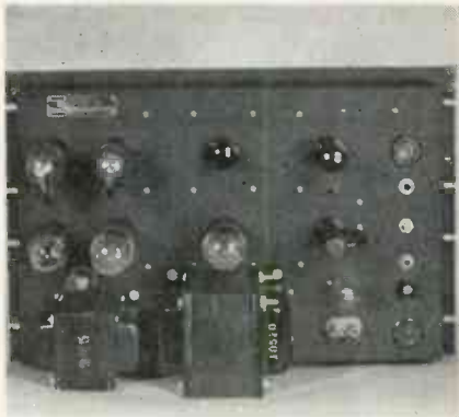
TUBES MOUNTED horizontally on reverse side of anemometer panel which is shown below at the right
