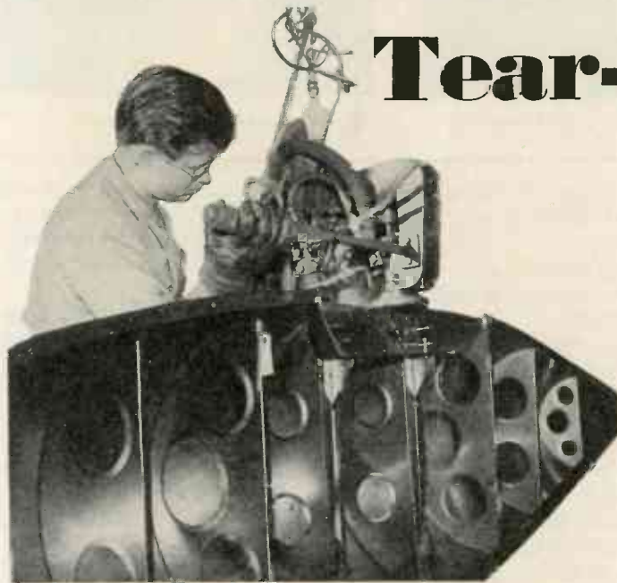
A PORTABLE SEAM welder operated in direction counter to movement of conveyor holding tank cuts welding time in half
