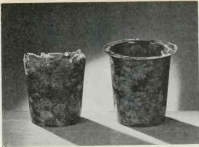
TEST CUPS molded of high impact-resistant phenolic material. Total pressure 16,000 lbs. Left: Standard Molded cup not filled. Right: Heatronic Molded 14 seconds close
