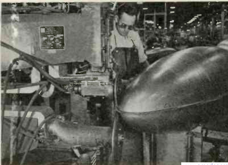
HALVES of the tank, spot welded together are supported in cradle as seam welder is run completely around to join them
