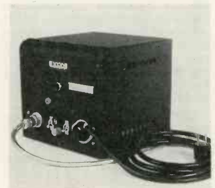
IMPULSE COUNTER constructed by R. J. Cashman for use with the Coblenz-Cashman-Rentschler phototube
