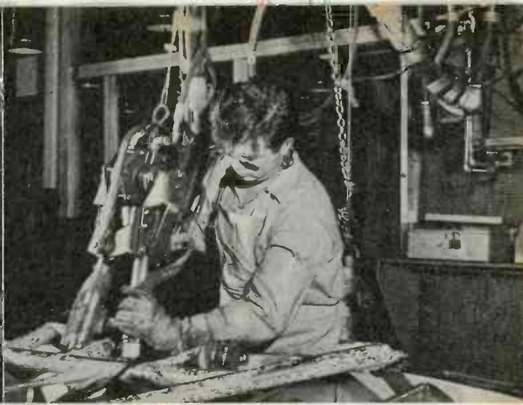
STRUCTURE SIMILAR to the keel of a boat is here spot welded to the tank while it is carried on a moving conveyor
