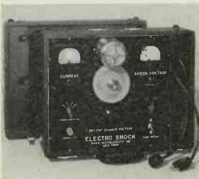
ELECTRO SHOCK therapy with self-contained recording surge current meter. Rahn Instruments, Inc., New York
