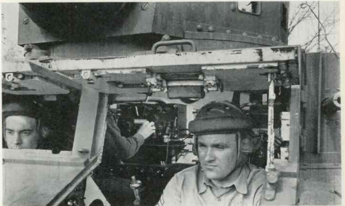
VITAL PART played by radio communication facilities in all phases of the war are emphasized in these two views showing typical installations behind the side gunner in an American bombing plane and in an M3 light tank
