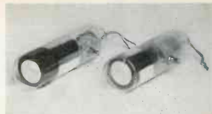
ULTRA - VIOLET Mg phototubes constructed for Bureau of Standards' W. W. Coblenz by R. J. Cashman, Northwestern University
