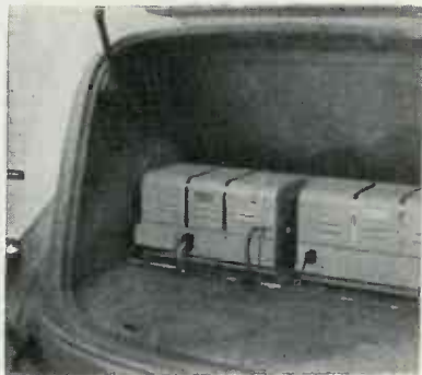
Complete 22 Watt High Frequency Mobile Installation
