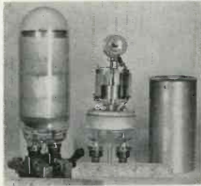
ILLUMINATION measuring unit. Weather Bureau mounts phototube, trigger tube, condensers and resistors inside frosted bulb filled with dry air
