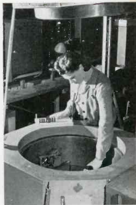
Temperature-control cabinet in which crystals are tested automatically, over the entire temperature range
