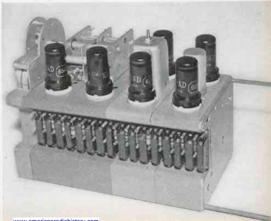
Flexibility of construction is shown in this four-cell communication receiver
