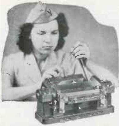
DI-ACRO Brake forms non-stock angles, channels or "Vees". Right or left hand operation. Folding width—Brake No. 1—6". Brake No. 2—12". Brake No. 3—18".
