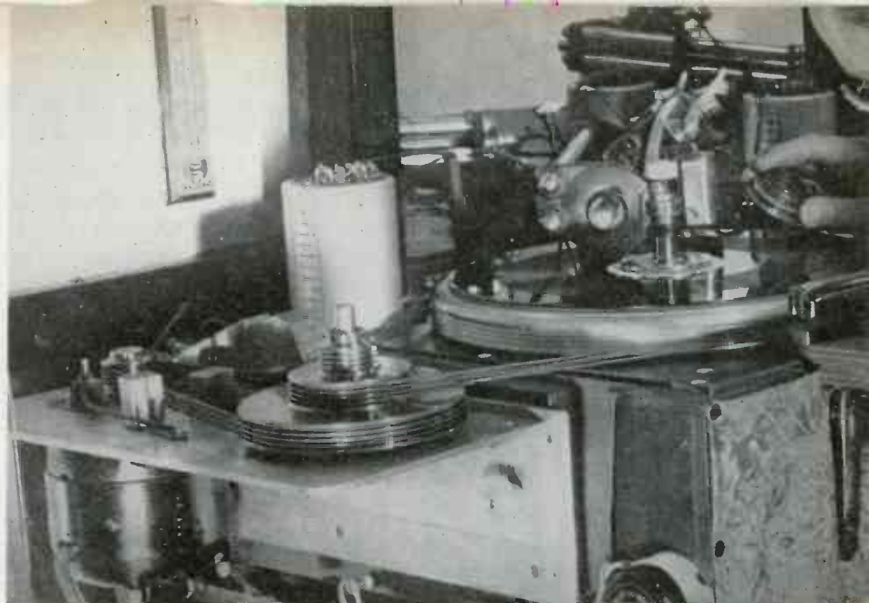
Fig. 2. Left-hand turntable, drive, motor, etc. Note the single belts passing around driver and driven members, making four pulling members, in each case
