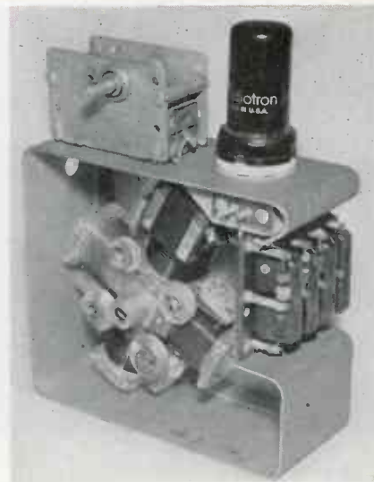
Close up of rf cell unit showing the four-band turret coil
