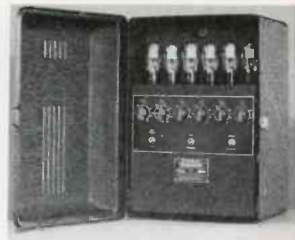
AUTOMATIC weld timer, NEMA type 5B, provides squeeze, weld interval, heat, cool, hold and off times, for spot or pulsation welding, repeat or non-repeat. Westinghouse model illustrated
