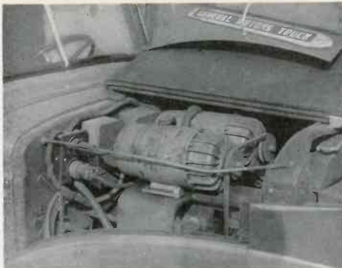
Above—Mobile unit generator (350-watt, 115-volt, 60-cycle each). At right—Interior view of WGAR mobile unit. 161.1-mc transmitter at center, mixer-audio amplifier on left, and 1622-kc receiver below
