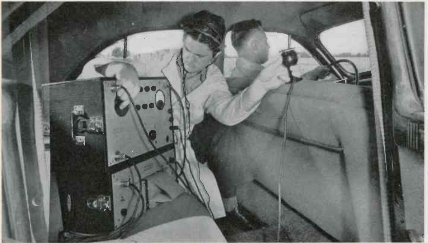
Recording the sound-frequency characteristics inside a closed sedan
