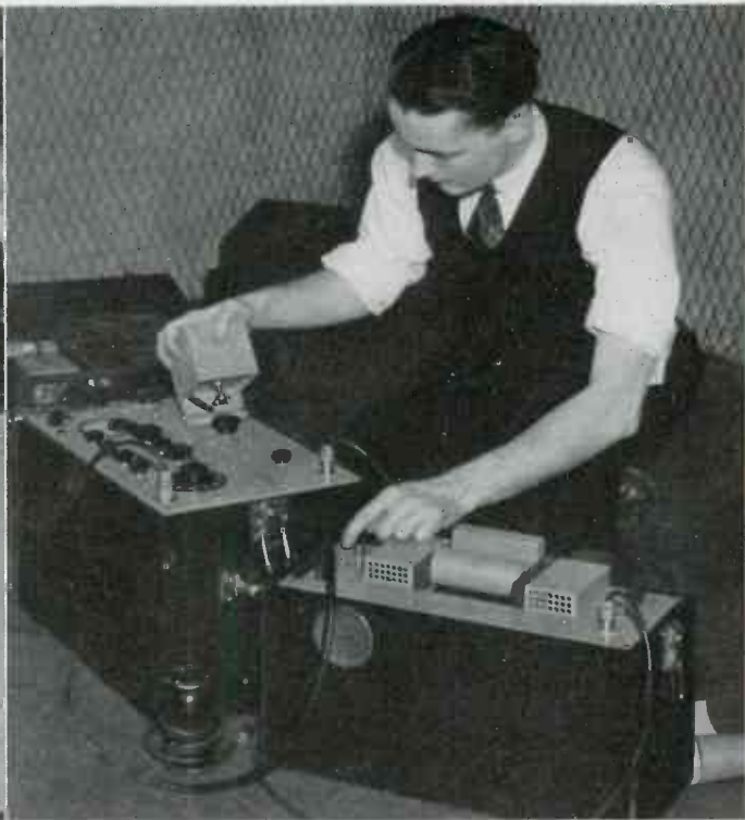
Analyzing the noise of an electric refrigerator in laboratory tests with a Western Electric recording sound frequency analyzer
