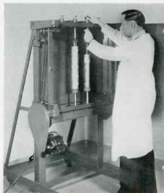
X-RAY jig to photograph 20 cylindrical aircraft engine connecting rod bearings in 10 min. instead of previous 5 hrs.
