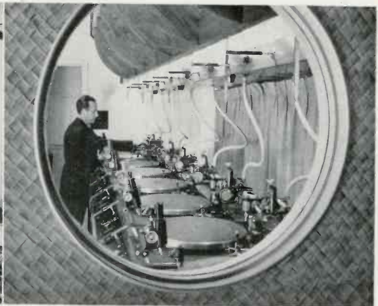
Reference recording room contains ten channels, for "recording off the line" or "off the air"
