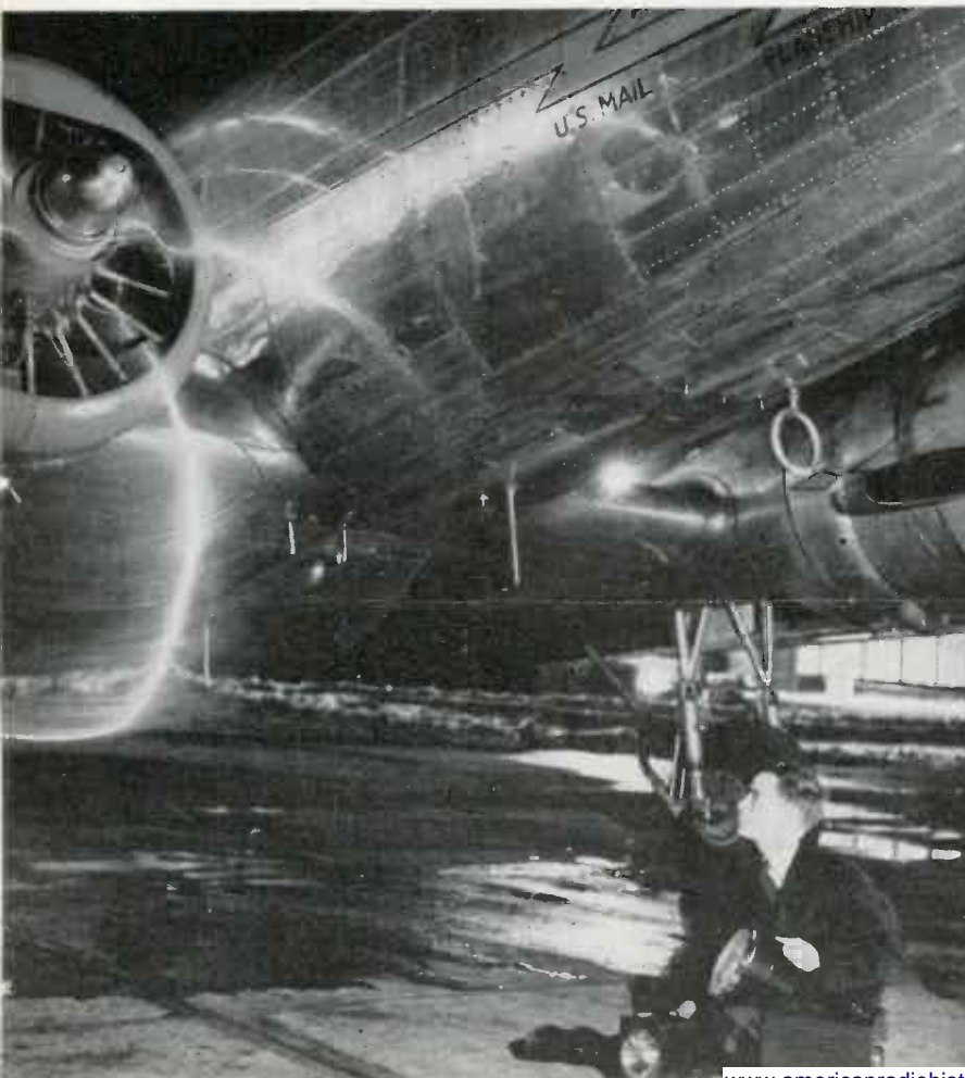
▼ PROPELLER at high speed studied in "slow motion" with General Radio stroboscope
