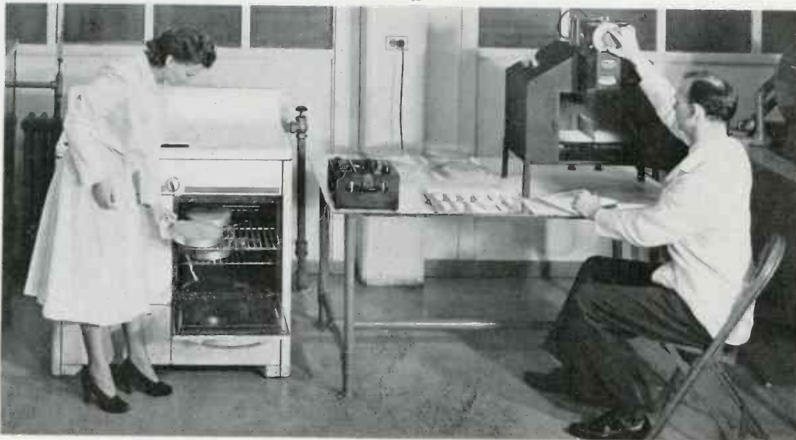
Exposing unit area of baked product to photocell measures oven efficiency
