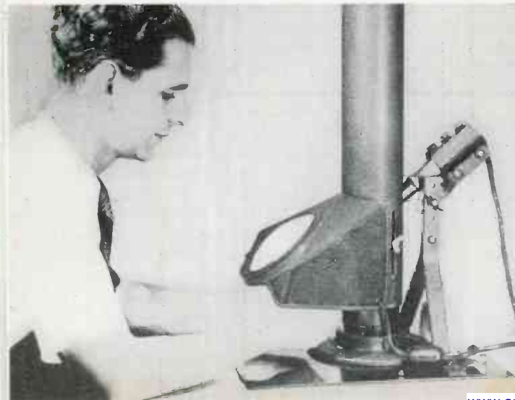
SOLDERING small, delicate parts is facilitated with this Photobell Corp. stand used by General Electric and other manufacturers. The unit consists of a holder for any standard size electric solder iron, hood and chimney to remove fumes, lamps and magnifying glass ▼ in hood to view work while held against solder iron
