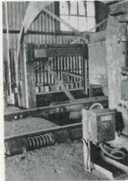
In foreground is housing photo-cell operated by beam across back
