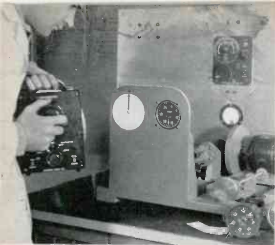
▲ TACHOMETER testing with General Radio stroboscope calibrated in flashes per min.
