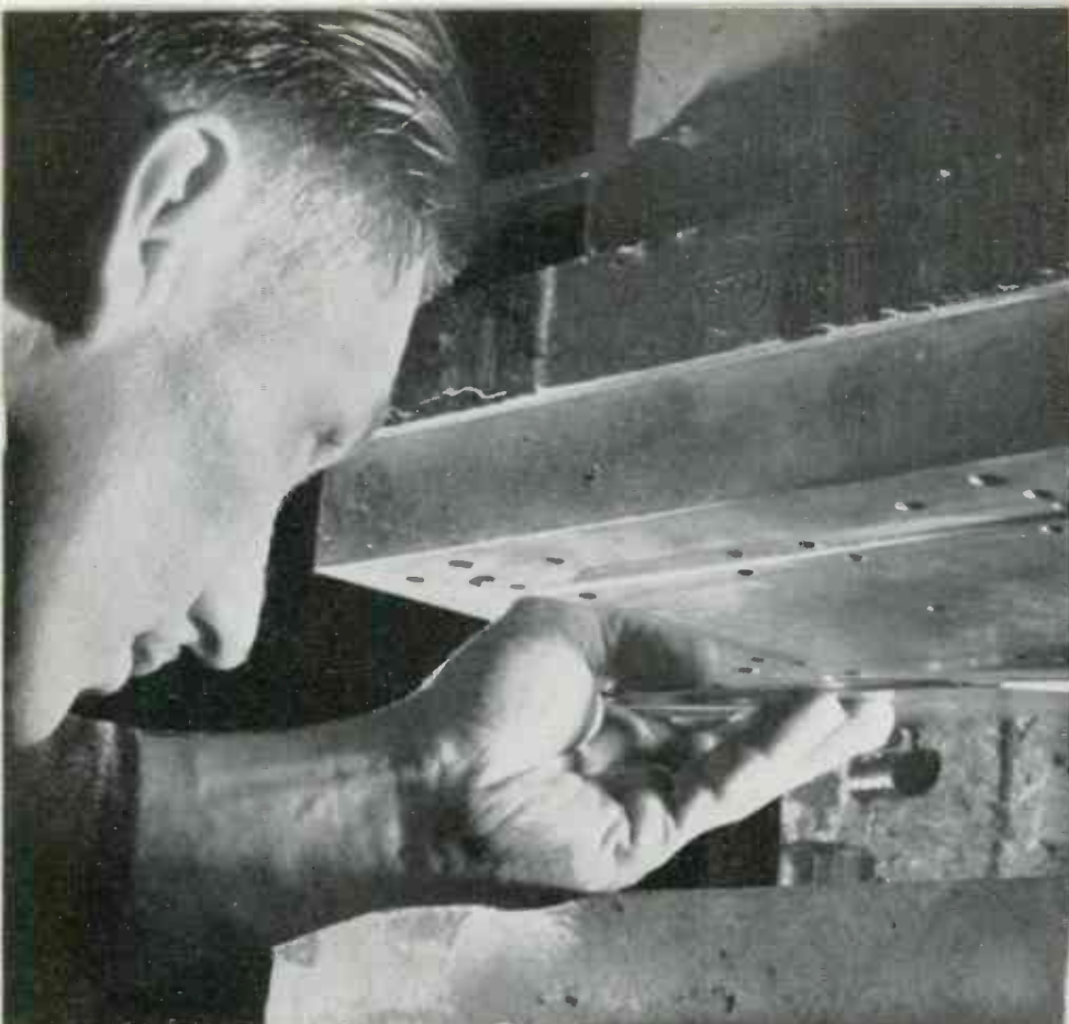
▲ AIR at 80 lbs. pressure blowing through upper die of Westinghouse punch press, supports stamped part in stream by pressure-velocity principle. Easy removal doubled output
