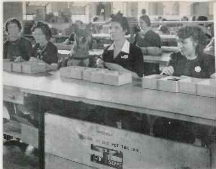
▲ BLIND workers' nimble, Braille-trained fingers sort mica sheets in West New York, N. J., plant of the Solar Mfg. Co., to within a few thousandths of an inch. Sheets from .002-.005 in. are accepted; others rejected
