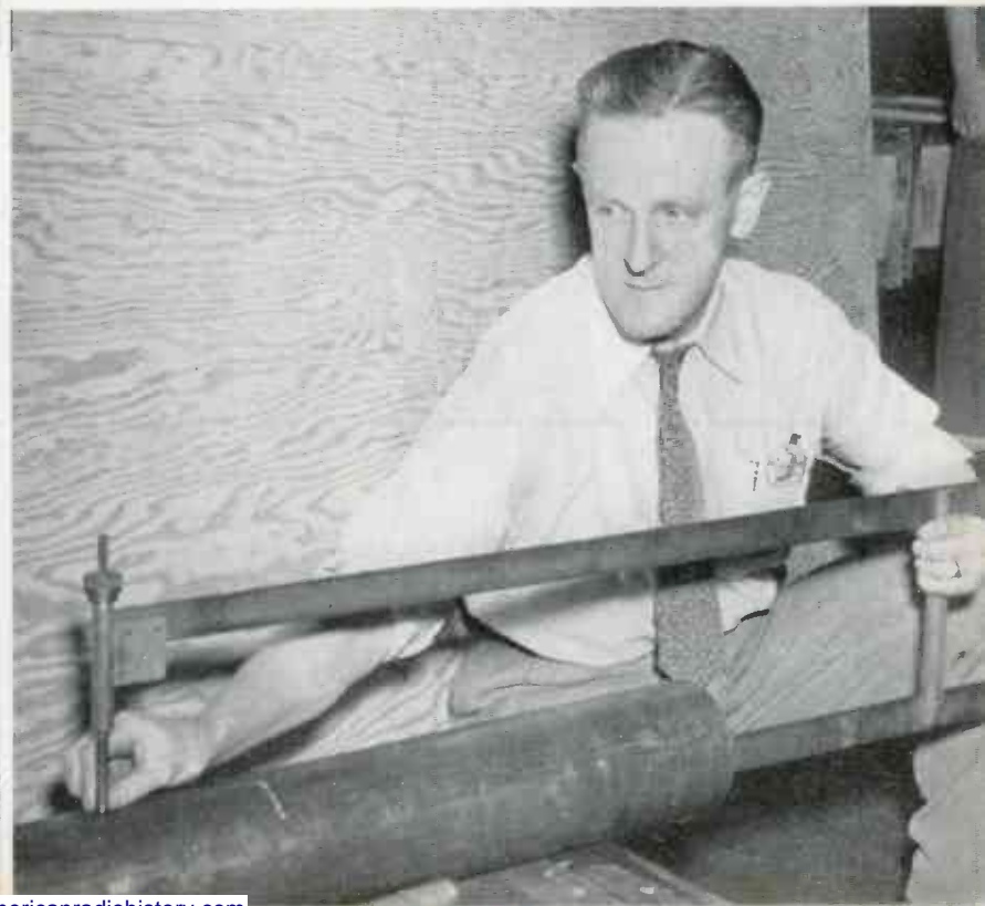
▼ CALIPER for determining wall thickness and relation of cored interior to surface prevents waste of man-hours machining defective castings. New caliper is demonstrated by Stanley Crawford, of RCA's Camden plant
