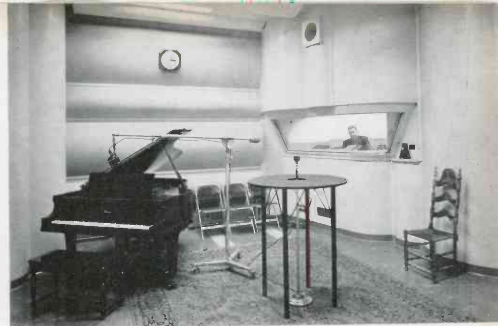
▲ End view of studio, with control room in the background. The back wall shows clearly the curved convex panels of different sizes, which disperse the sound. Note also shelf-enclosed microphone, which is non-directional, and is held at a convenient distance from speakers
