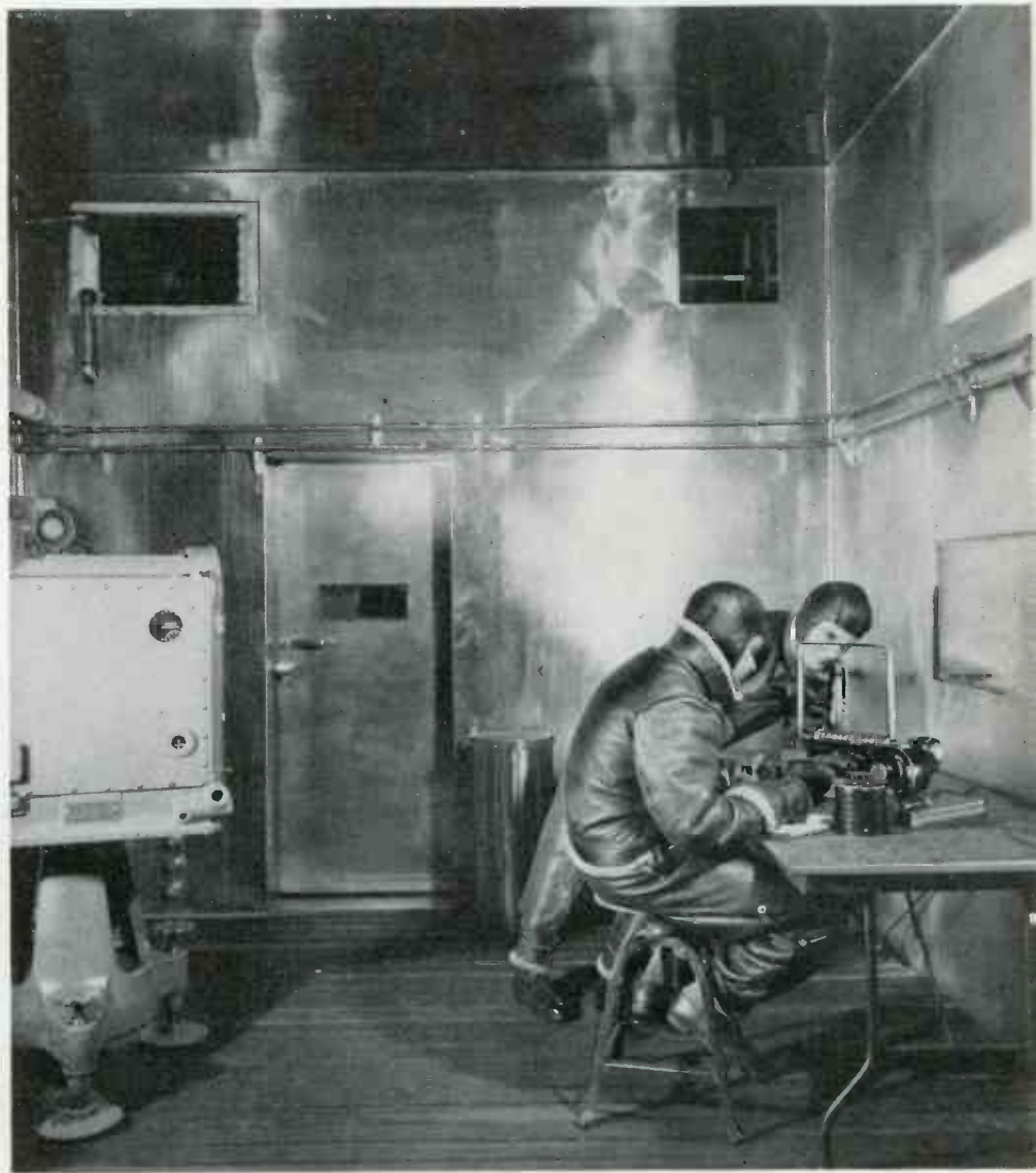
▲ TEST-ROOM in the laboratory of the Sperry Gyroscope Company, Brooklyn, N. Y., used for simulated flight testing of a variety of electronic equipment for aircraft. The room is eleven feet square, ten feet high, and consists of a "floating" shell of stainless steel to resist fresh and salt-water simulated fogs, powerful ultra-violet light radiation, or simulated rain. The Tenney steel room is suspended at the center of the ceiling and floats in eight-inch insulation, with sliding fits at observation windows and doors. The shell is anchored at a central drain in the floor. A five ton refrigerating system maintains room at zero; temperatures to -40^{\circ}\text{F} . are achieved with dry ice. Chamber can be heated to 150^{\circ}\text{F} . Humidity may be controlled from apparatus dew point to 95%
