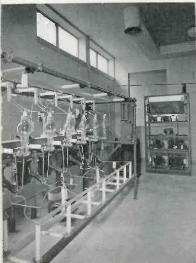
Doherty final amplifier. Tube on left is peak tube, tube on right is the → carrier tube. The output of the amplifier feeding the antenna system, is 50 kw
