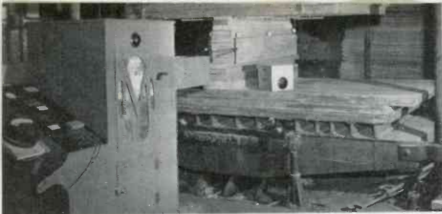
▲ EDGE-GLUING plywood propeller blanks with 12 mc electrostatic heating by Mann and Russell "parallel bonding" process in which lines of force follow glue layers in Wheeler Osgood Co. plant at Tacoma, Wash.
