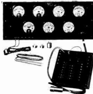
Pattern 579 Service Test Panel
