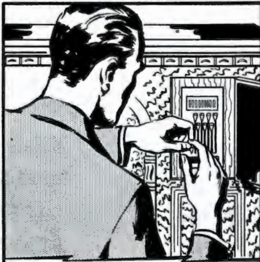
You lock this tuning on the first Zenith Automatic button, without tools, by merely loosening the button, depressing the arm and tightening the button again, and mark the name of the station in the first space on the card.
