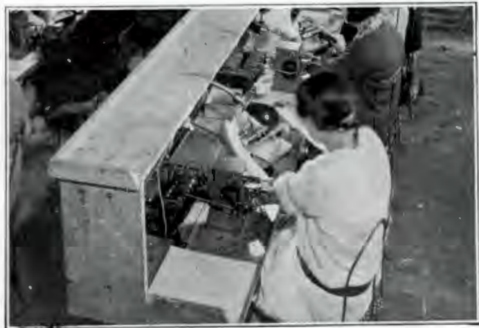
SPOT-WELDING ON THE very small units of a radio tube requires concentration and skill. Thoroughness is essential in this work, and it is accorded by these young women.
