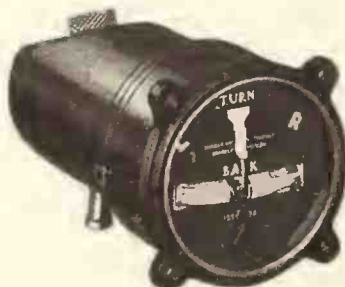
Turn and Bank Indicator used in conjunction with Earth Inductor Compass.
