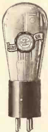
Type GSX-213 Rectifier tube, designed to accomplish full wave rectification of alternating current (a. c.) to direct current (d. c.) List price $5.00
