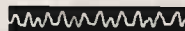
Sound-photograph of phonograph reproduction—exposure one-twentieth of a second. In the absence of detail appears the cause of that "phonograph tone" universally recognized as characteristic of all phonograph music.
