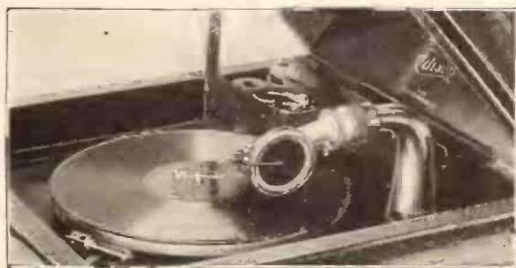
Showing Convenient Position of Reproducer When Changing Needle
