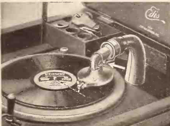
SHOWS POSITION FOR PLAYING EDISON AND OTHER VERTICAL CUT RECORDS
