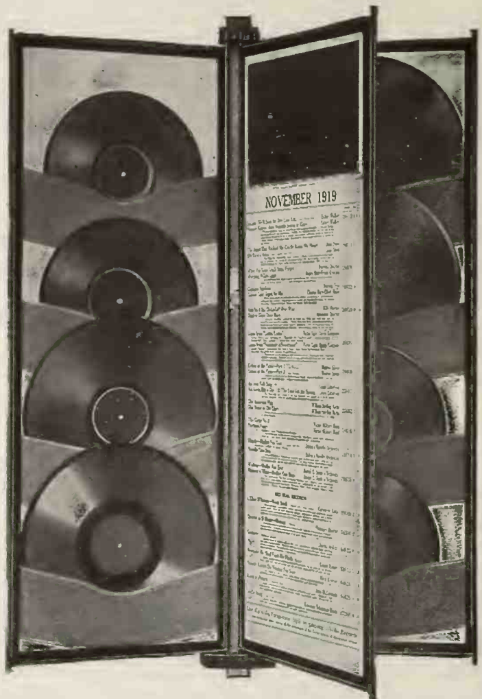
No. 562. Universal Combination Self-Service and Bulletin Wall Displayor, equipped with three wings, 13x36 inches, 16 pockets for holding 10 or 12-inch records and two monthly bulletins. Can be attached to wall or inside your demonstration booth. Projects only four inches when not in use. Constructed of steel channel frame with 1/4-inch steel rod on the outside, electrically welded, finished in double-baked ebony enamel. Wings swing from left to right or right to left. Has patented locking device at the top to prevent leaves from coming out.
