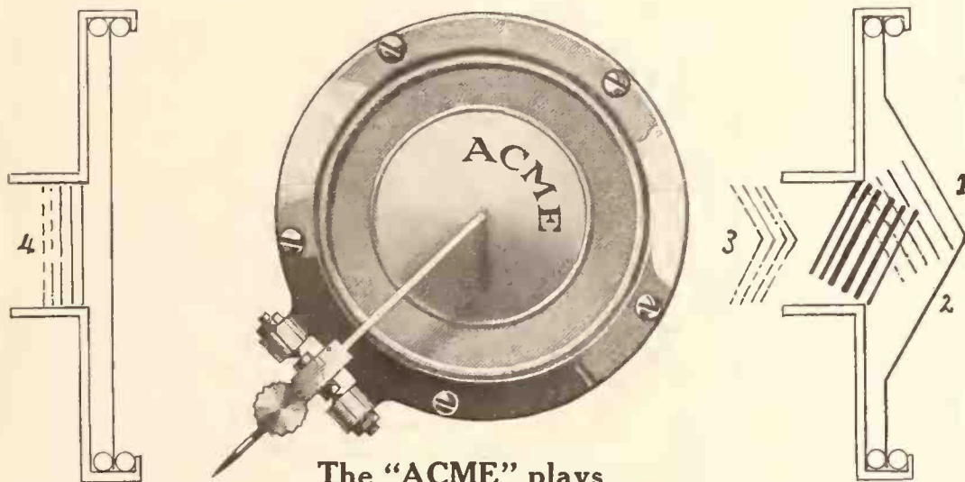
This illustration shows the short tone waves of the ordinary soundbox as used on most phonographs.
