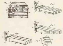
structed in accordance with this invention; Figs. 3 and 4 are perspective views of two different forms of sound amplifiers constructed in accordance with this invention; and Fig. 5 is a longitudinal horizontal section of a sound amplifier constructed in accordance with this invention.
