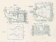
tical central section of a talking machine constructed in accordance with this invention; Fig. 2 a top plan view of a portion of the same, and Figs. 3 and 4 are a top plan view and a fragmentary front elevation, respectively, of the machine with parts removed.
