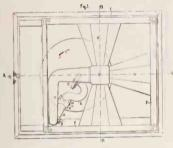
The invention further consists in pivotally connecting the portion of the sound pipe which carries the sound box to the rest of the sound pipe in such a manner that the two portions of said sound pipe are coaxial at the joint in their normal working position, and whereby the gradual taper of the sound pipe may be continued to the sound box itself.
