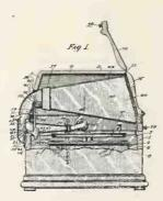
The main objects of this invention are: to provide a compact inclosed talking machine; to provide a talking machine in which the amplifier, the record support, and the actuating mechanism for the record support are inclosed in a cabinet provided with a movable eover. and in which the
