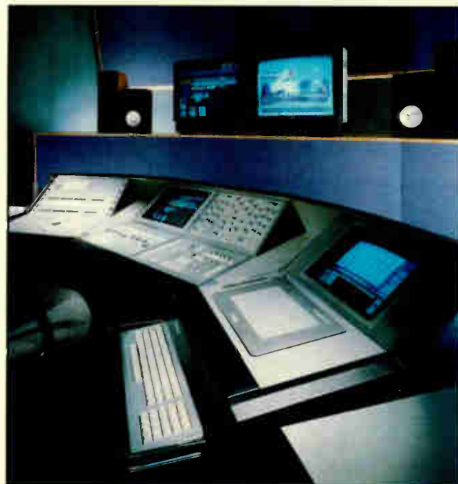
The Scenaria has 24 digital I/O's and 32 analog.
