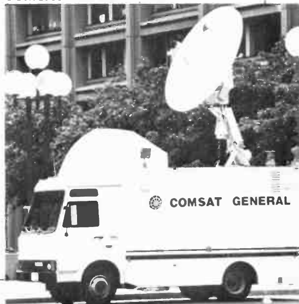
COMSAT's mobile SNG unit
