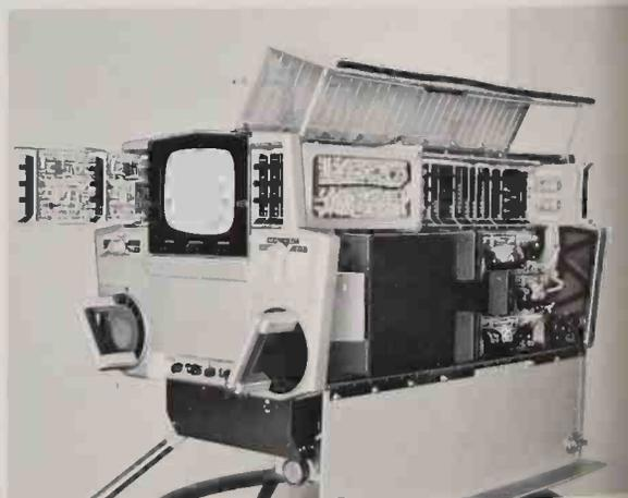
*Plug-in transistorized modules speed servicing, increase reliability.*
