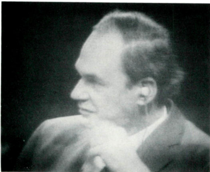
Figure 19: TV picture with 50 dB down interfering signal.
