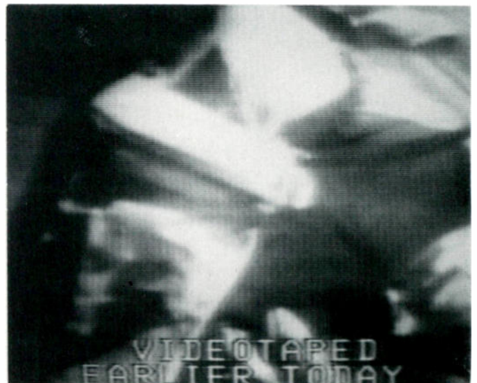
Figure 17: TV picture with 40 dB down interfering signal.
