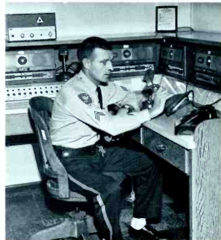
On duty at the police building in downtown St. Mary's, Sergeant James H. May keeps in touch not only with police cars in his own city, but with vehicles in all towns in the county. Remote control units at the desk console, provided by General Electric, maintain instant contact through the entire system network.
