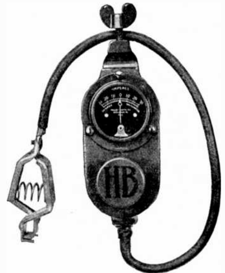
A compact battery charging control. The ammeter shows what current is being taken and the intensity of the current is regulated by turning the knob directly below the dial. This operates upon a pressure rheostat.
