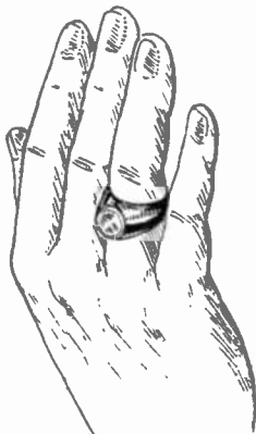
An illuminated dial compass mounted seal ring fashion, primarily for electrician's use. The magnetic needle is a detector of currents and the illuminated dial feature makes the ring useful in obscure corners and dark places.
