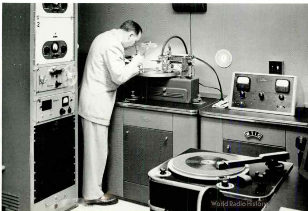
▼ New technology comes to WTIC. This photo shows the transition of recording techniques. The equipment at left includes a newly purchased tape recorder. Engineer Al Jackson checks a transcription disk — the old recording method.
