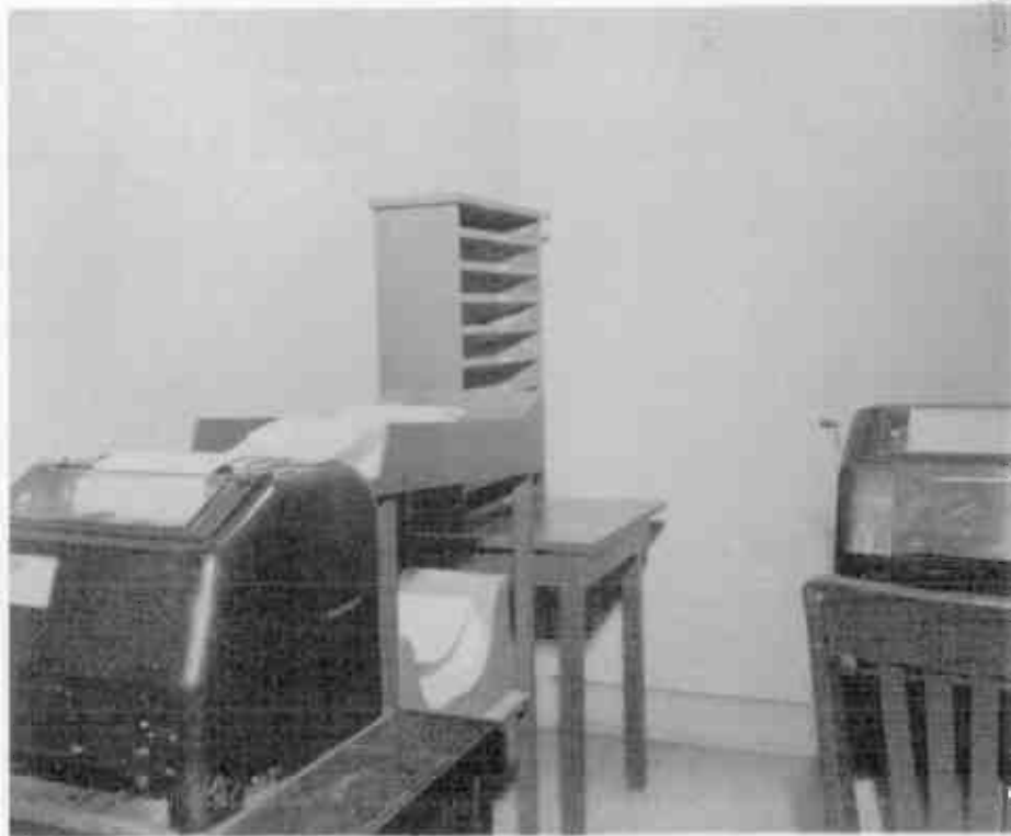
A portion of the WSJS teletype room, showing (at left) the kind of machine on which United Press news is automatically written from a leased wire for 19 continuous hours each day. The copy paper is drawn from the lower rack behind the machine and deposited in the upper shelf, then sorted by WSJS news men into the rear cabinet.
