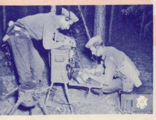
Portable Army radio outfit operates on maneuvers. Note hand generator.
