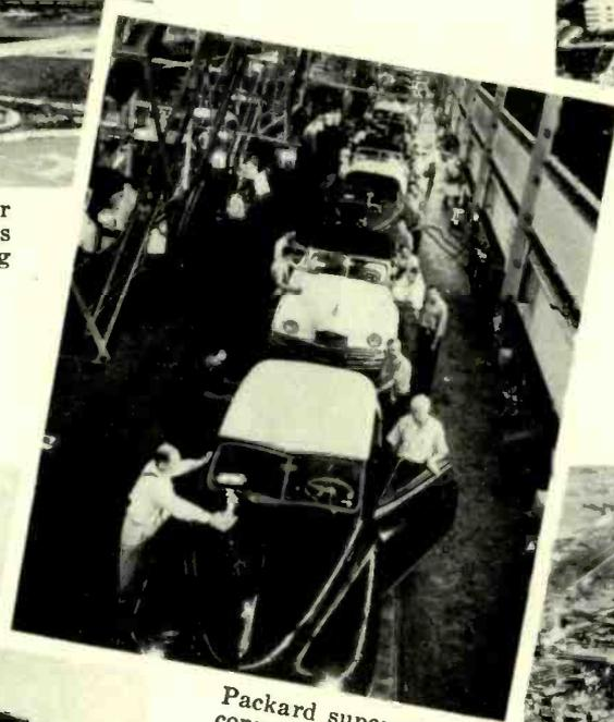
Packard super eight convertibles moving down one of the two assembly lines at the Packard Motor Company plant in Detroit.
