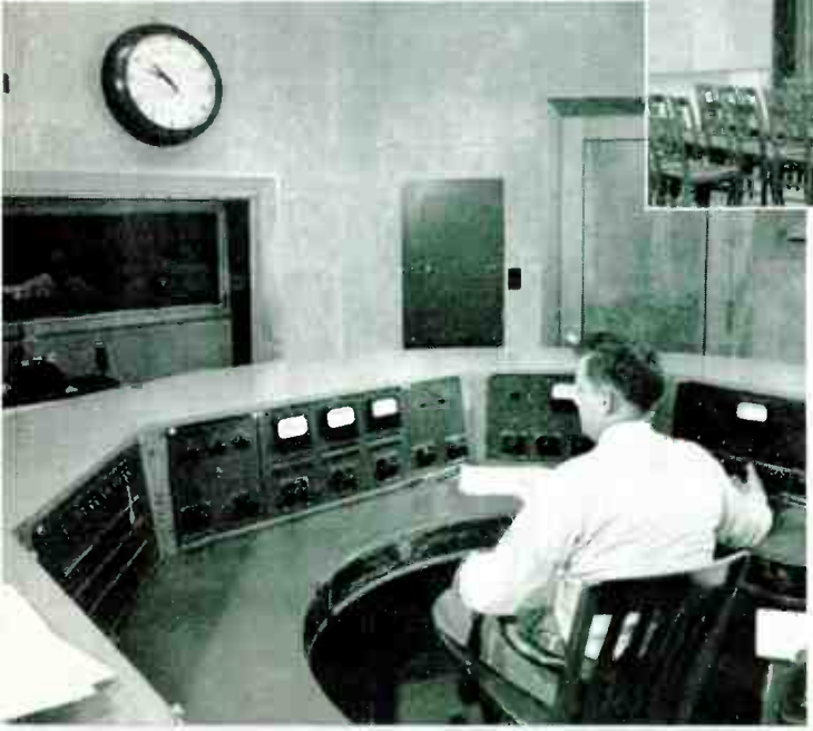
Master Control Room . . . and amplifying racks, slightly elevated to command a view of all studio operations and to feed the NBC network broadcasts.
