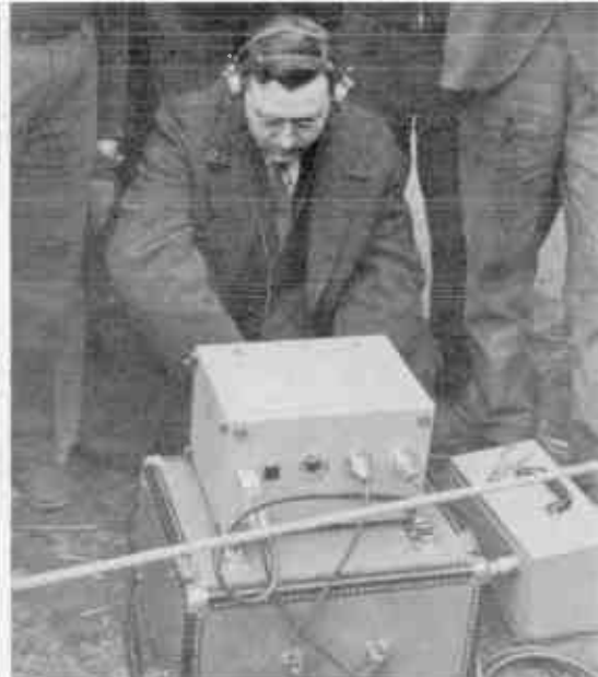
Behind All WBCM "Special Events" is the remote-control staff of WBCM engineers. Chief Engineer Ralph Carpenter is shown here with the portable amplifier, at the Ridotto fire. Microphone lines lead into the amplifier before him, where volume is regulated and additional electrical current is applied to "boost" the sound to the transmitter.
