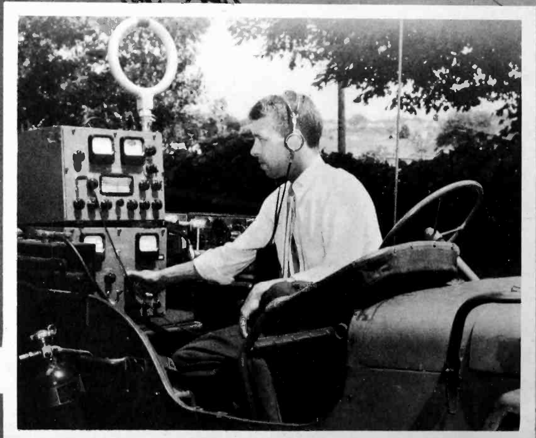
WAGE's chief engineer CHARLES BRANNEN uses a jeep in field tests to measure WAGE's signal strength.
