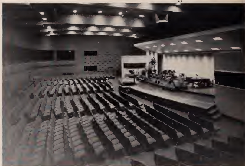
Radio City's world-famous Studio 8-H recently underwent extensive face-lifting. Here is the redecorated studio equipped with a new "sound box" stage and other acoustical properties including sound absorbing upholstered chairs.
