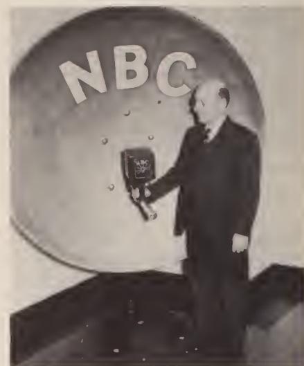
Gustave A. Bosler is shown next to a six-foot parabola microphone with which field engineers can, from the grandstands, pick up the crack of the bat hitting the ball or the thud of the ball in the catcher's mitt during a ball game.
