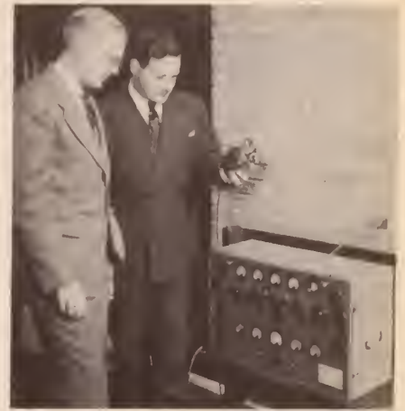
NBC San Francisco has acquired a new portable transmitter which is especially designed for use in airplanes. Here are Western Division Engineer A. H. Saxton, and Curtis Peck, engineer in charge of the San Francisco studios, inspecting the new, 100-watt transmitter, which weighs only 100 pounds.
