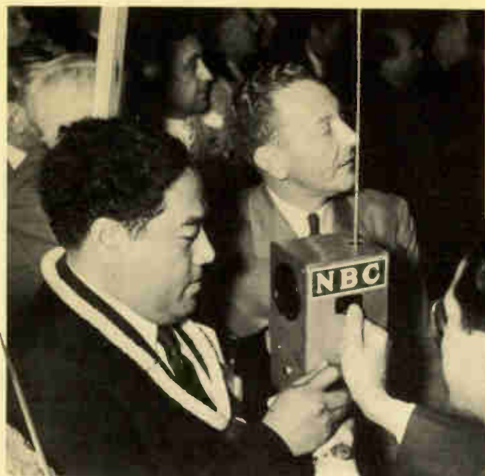
NBC's Chief Engineer, O. B. Hanson, demonstrates the first model of the micro-wave transmitter, the midget radio station. Concealed in a top-hat, the transmitter has its power supply in batteries worn in a belt. A later model ( left ) built in a box with a handle, was widely used during NBC broadcasts from 1936 political conventions.
