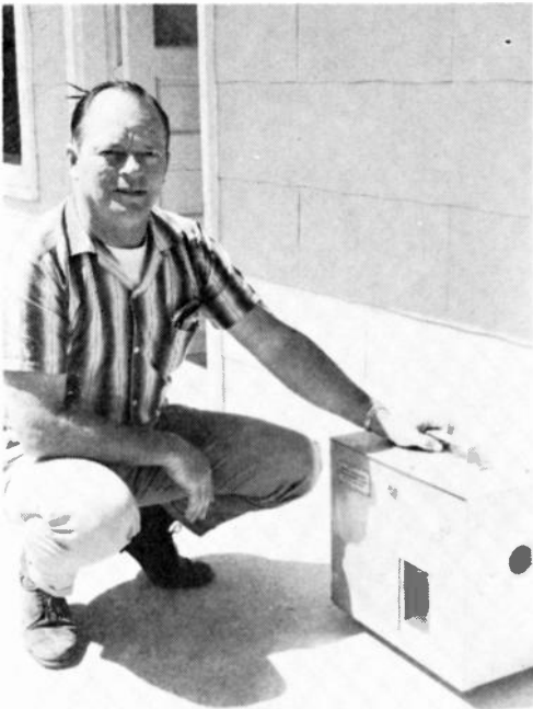
Jack Gowing inspects generator in which silver iodide is burned at 2300 degrees for the purpose of seeding the clouds.
