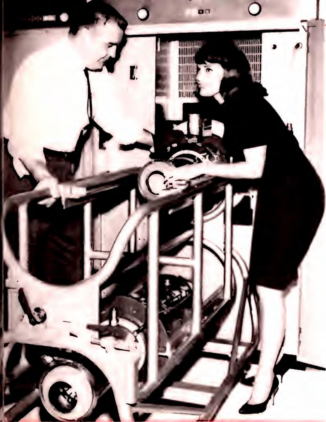
RCA's recently introduced vapor-cooled klystron UHF transmitter is demonstrated by Tom Mullooney (l), of the broadcast and communications products division, and Anita Eurbank of Northwestern University. The 250-pound tube slides out onto a specially-designed carriage that revolves to permit a fresh tube to be placed into position.
